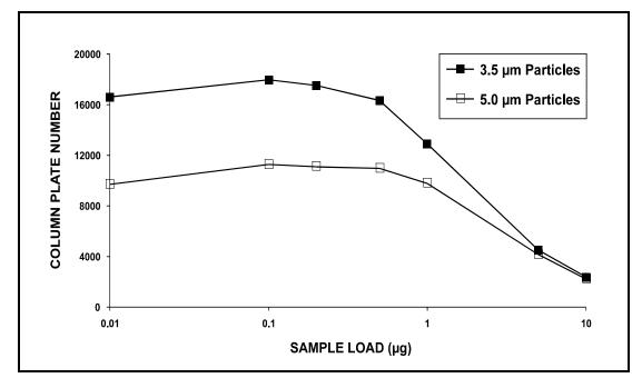
ZORBAX<sup>®</sup> SB-C8 (3.5 µm and 5 µm) (4.6 x 150 mm) (P/N:863953.906 and 883975.906)
