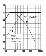
When combined with an 6" or 8" acoustic suspension, 2 way system
