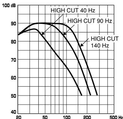
The figures below show the optimum adjustment of each control and the frequency characteristics when this subwoofer is combined with a typical main speaker system.
