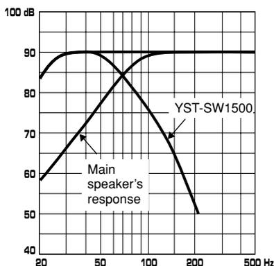
**EX.2 When combined with an 8" or 10" (20 cm or 25 cm) acoustic suspension, 2 way system main speakers**
