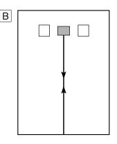
It is recommended to place the subwoofer on the outside of either the right or the left main speaker. (See fig.  $\boxed{A}$ .) The placement shown in fig.  $\boxed{B}$  is also possible, however, if the subwoofer system is placed directly facing the wall, the bass effect may die because the sound from it and the sound reflected by the wall may cancel out each other. To prevent this from happening, face the subwoofer system at an angle as shown in fig.  $\boxed{A}$ .
