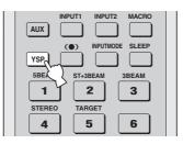
**6** Press one of the beam mode buttons to select the desired beam mode. For further details about the beam modes, see page 42 in the supplied Owner's Manual.
