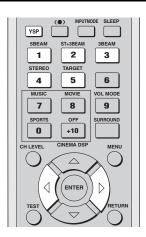
1 Press YSP on the remote control to switch to the operation mode of this unit.
