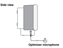
Place the optimizer microphone on a flat level surface more than 2 m from the front of the unit and within 1 m from the center height of the unit with the optimizer microphone head upward at your normal listening position.
