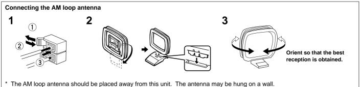
The Aivi loop antenna should be placed away north this unit. The antenna may be hung on a wall.
