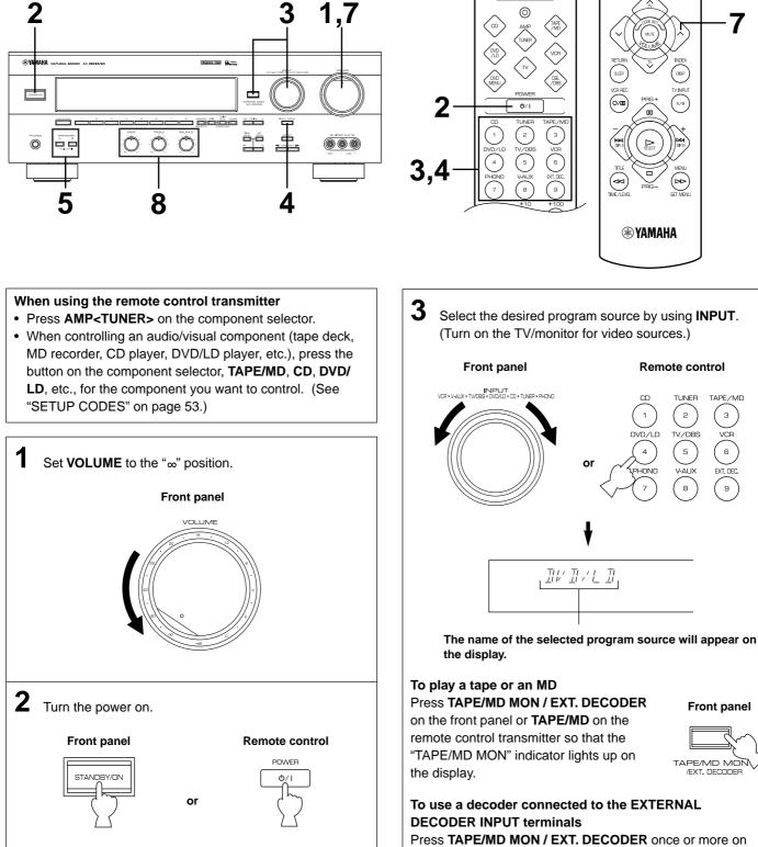
Press **TAPE/MD MON / EXT. DECODER** once or more on the front panel or **EXT. DEC.** on the remote control transmitter so that "EXT. DECDR" appears on the display.
