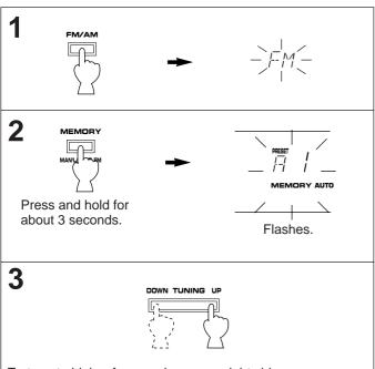
To tune to higher frequencies, press right side once. To tune to lower frequencies, press left side once.
