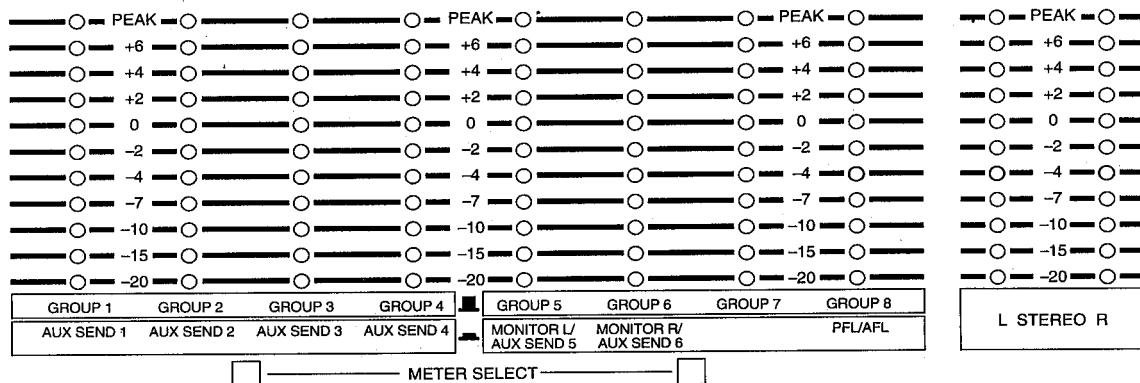
RM800 features ten 11-segment LED meters, providing output level metering for all outputs. The STEREO meters are dedicated to the stereo output, whereas the GROUP meters are dual operation meters. The METER SELECT switches are used to select which signals are displayed. The following table shows how they work.
