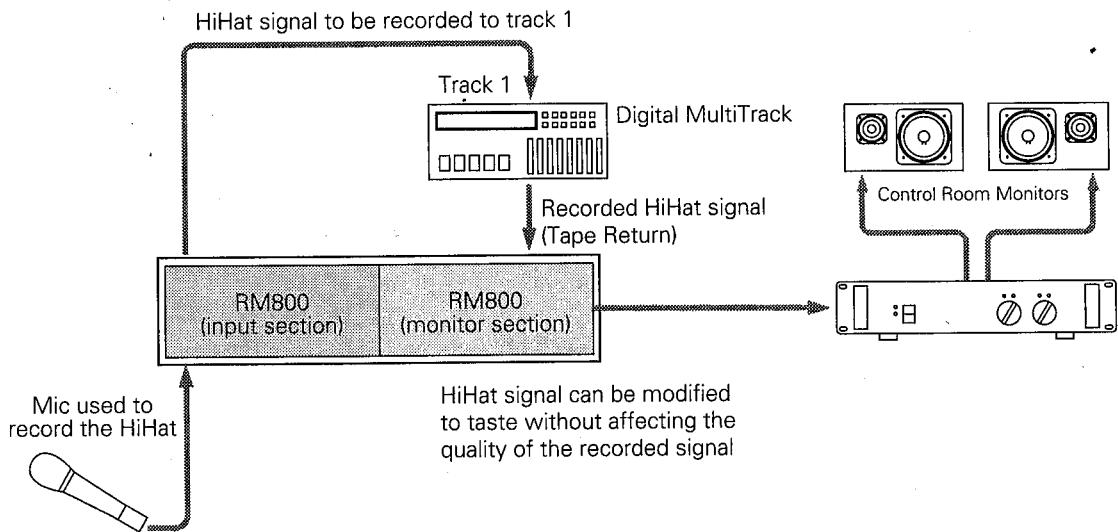
On an in-line console, multitrack *playback* can be mixed as required using the 'monitor section' of a channel module, while the input fader, EQ etc. positions are set to optimize signal level on each track of the recorder.
