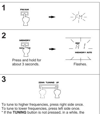
\* If the TUNING button is not pressed, in a while, the
