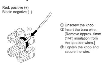
Banana Plug connections are also possible. Simply insert the Banana Plug connector into the corresponding terminal.
