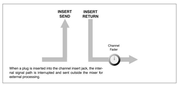
Channel insert jacks must be used with a special insert cable that has a TRS phone jack on one end and mono phone jacks on the split "Y" end. One of the mono phone jacks carries the "send" signal to be fed to the input of the external processor, and the other carries the "return" signal from the output of the processor.
