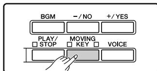
While holding down the [MOVING KEY] button, press the highlighted keys shown below to check the version number and select the part (channel) for the Moving Key feature.
