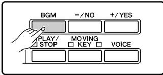
While holding down the [BGM] button, press the highlighted keys shown below to adjust transposition, touch sensitivity, and switch the song auto revoice on/off.
