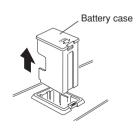
4 Slide the battery case back into the battery holder and press firmly so that the battery case locks into place.
