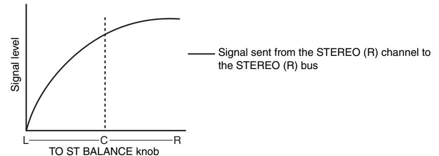
If the CSR knob is set to 100%, operating the INPUT TO ST PAN knob will change the level of signals sent to the STEREO (L/R) bus and MONO (C) bus, as shown in the following diagram.
