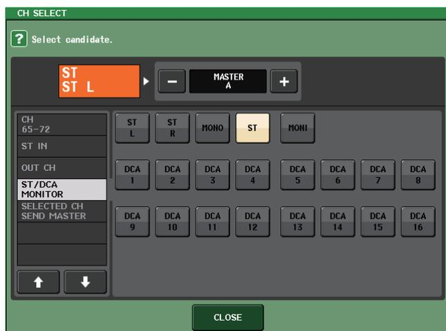
Use the list in the left column to select the desired channel group, then use the buttons in the right column to select channels. When you have finished selecting the channels, press the CLOSE button.
