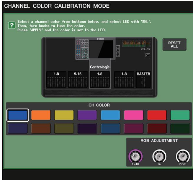
3. Press a [SEL] key on the top panel to select the indicator for which you want to adjust the color.
