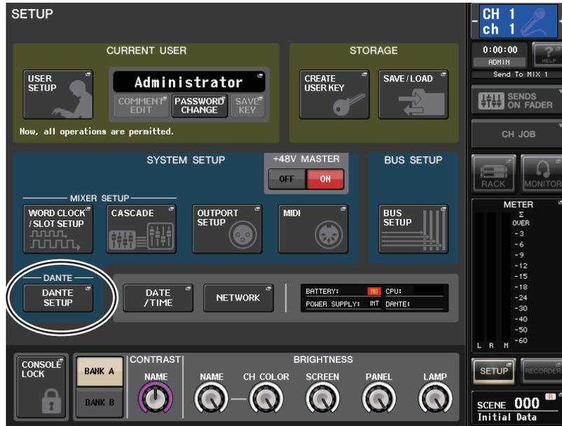
2. In the **DANTE** field at the center of the screen, press the **DANTE SETUP** button to open the **DANTE SETUP** popup window.
