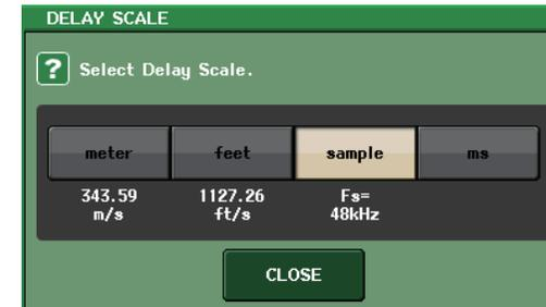
You can select one of the four delay scales: meter (meter/sec), feet (feet/sec), sample (number of samples), and ms (millisecond).
