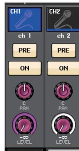
If the send source is stereo, you can use the PAN/BALANCE mode setting in the TO STEREO/MONO popup window to select whether PAN/BALANCE will function as a PAN or BALANCE knob.
