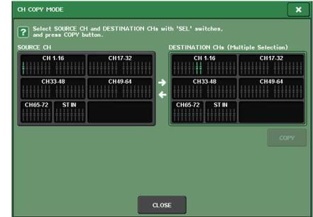
If the copy source is a MIX/MATRIX channel, buttons will appear so you will be able to select parameters to copy.
