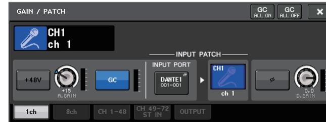
4. Use multifunction knob 8 to adjust the D. GAIN parameter.
