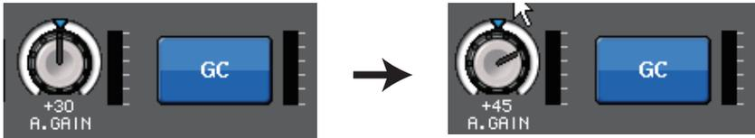
At this time, the gain of each signal input to the CL series unit will be adjusted by the digital gain parameter. If the FOH console and the monitoring console are sharing one I/O rack, adjusting the analog gain on the FOH console will not affect the input level on the monitoring console, because the level of the signal on the audio network is maintained at a constant level.
