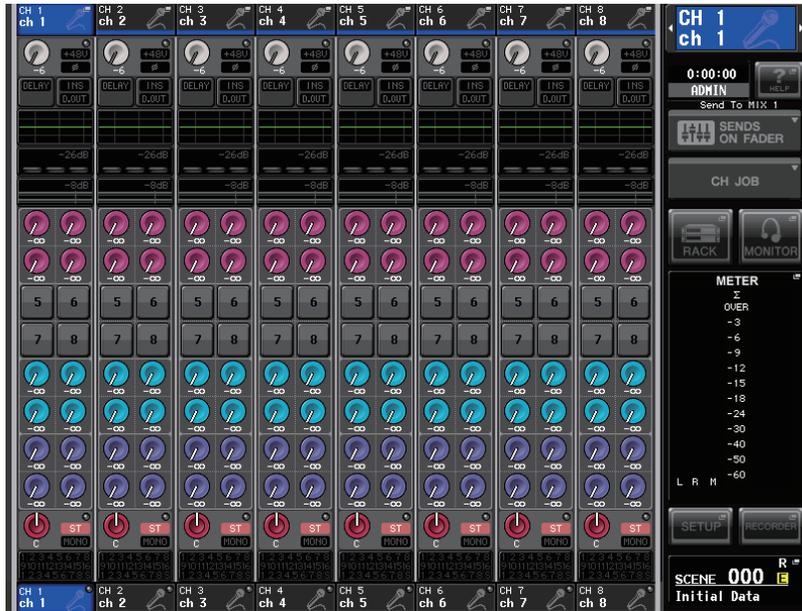
3. Press the TO MIX/MATRIX SEND LEVEL knob for the desired send-destination MIX/MATRIX bus.
