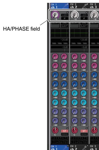
9. Press the PATCH button, and select the input port assigned to the external HA. With these settings, you will be able to use the external HA in the same way as the head amp on the I/O rack or the CL unit. For details about the GAIN/PATCH popup window, refer to “[Making HA \(Head Amp\) settings](#)” on page 30.
