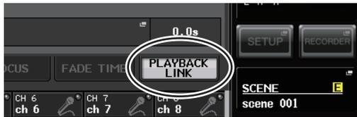
**3.** Press the PLAYBACK LINK tab at the bottom of the SCENE LIST window.
