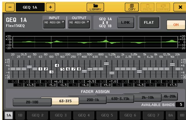
This window is the same as that for the 31BandGEQ, except that the AVAILABLE BANDS parameter box indicates the real-time number of additional bands (maximum 15) that can be controlled in the current GEQ.
