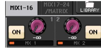
If necessary, you can specify two adjacent odd/even-numbered MIX/MATRIX buses as a stereo bus and link the main parameters.
