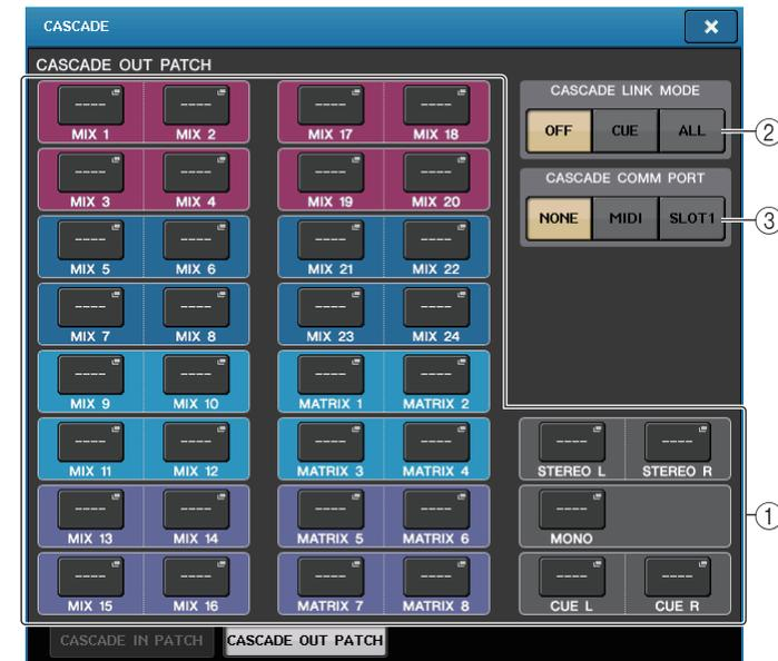
**① OUT PATCH buttons (CASCADE OUT PATCH section)**
