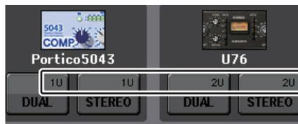
The U76 occupies two rack spaces. Other processors occupy one rack space. If you mount a two-space Premium Rack processor in the rack, you will be unable to mount any more processors below those rack spaces. Also, you cannot mount a two-space processor in Rack 8.
