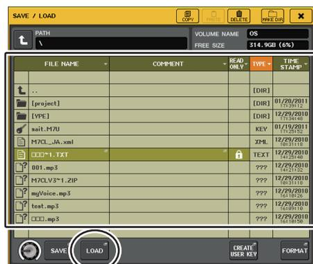
3. To select the file that you want to load, press the name of the desired file in the file list, or rotate the corresponding multifunction knob on the panel. The highlighted line in the file list indicates the file that is selected for operations.
