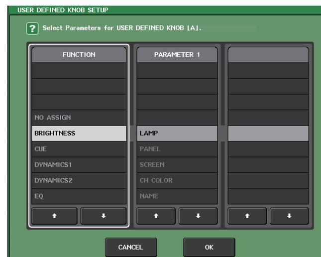
5. Make sure that the **FUNCTION** field is enclosed by a frame, then use the **↑/↓** buttons in the lower part of the field or the multifunction knobs on the top panel to select the function you want to assign.
