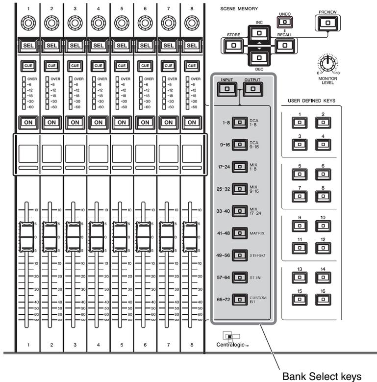
If you press one of the Bank Select keys, the channels or DCA groups corresponding to that key will be assigned to the Centralogic section, and can be controlled using the faders, [ON] keys, and [CUE] keys in the Centralogic section.
