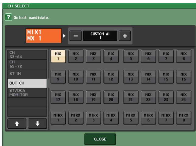
Use the list in the left column to select the desired channel group, then use the buttons in the right column to select channels.
