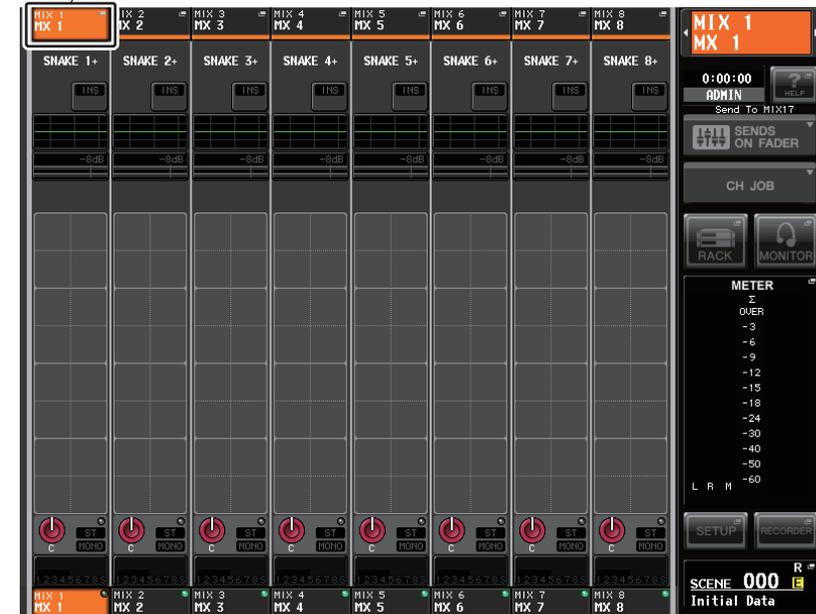
2. Access the PATCH/NAME popup window by pressing the channel number/channel name field of the channel to which you want to assign the channel name and icon.
