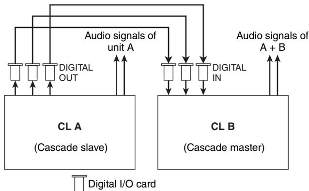
In this example, up to twenty four buses chosen from MIX bus 1–24, MATRIX bus 1–8, STEREO bus (L/R), MONO (C) bus, and CUE bus (L/R) can be shared, and the mixed signals transmitted from the cascade master CL unit. (If you use three 16-ch digital I/O cards, all buses can be shared among the devices.)
