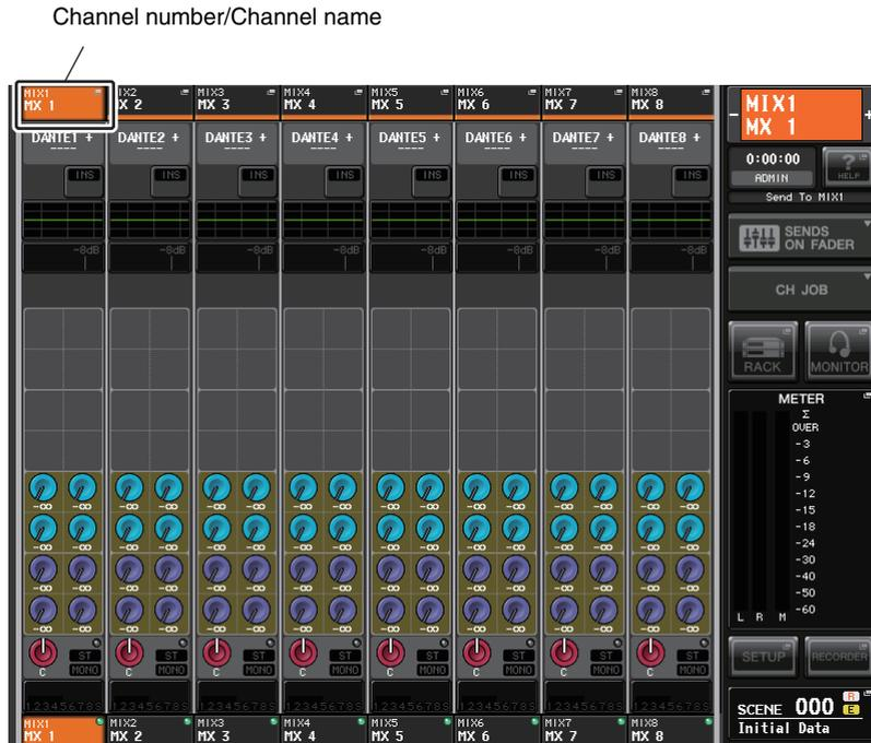
2. In the top part of the screen, press the channel number/channel name field to access the PATCH/NAME popup window.
