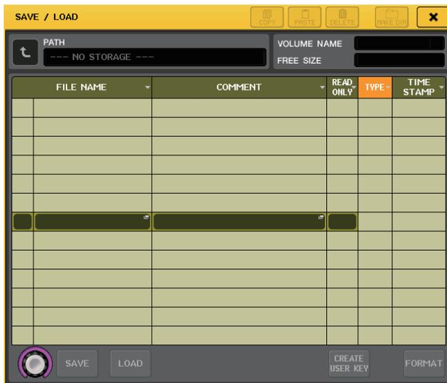
4. To select the Help file (file extension: .xml) that you want to load, press one of the Help files in the file list, or turn the multifunction knob on the panel.
