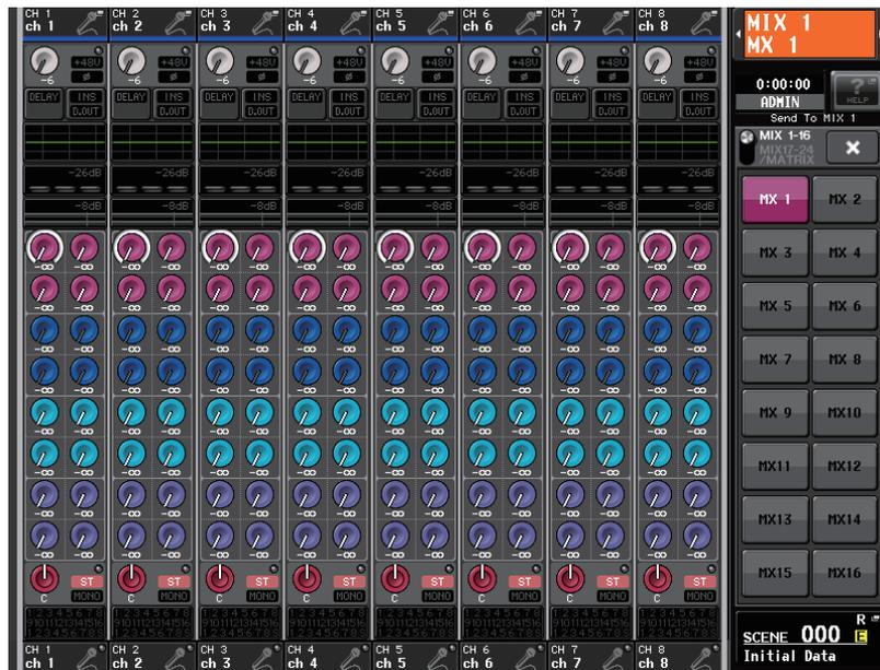
3. Press the MIX/MTRX ON FADER switch button repeatedly to select MIX1–16 or MIX17–24/MATRIX.
