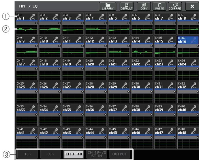
This window displays the corresponding input channels (or output channels) simultaneously. This page is only for display, and does not allow the parameters to be edited. It is useful when you need to quickly check multiple EQ settings, or when you want to copy and paste EQ settings between distant channels.
