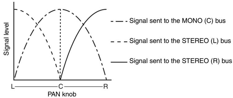
Operating the TO ST BALANCE knob of an ST IN channel will change the level of signals sent from the STEREO L/R channels to the STEREO (L/R) bus and MONO (C) bus, as shown in the following diagram.
