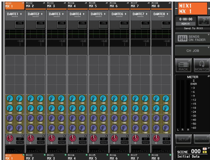
3. Press the TO MATRIX SEND LEVEL knob for the desired send-destination MATRIX bus.
