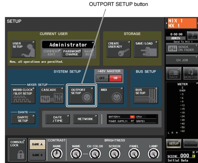
**2. In the SYSTEM SETUP field located in the center of the screen, press the OUTPUT SETUP button to open the OUTPUT PORT popup window.**
