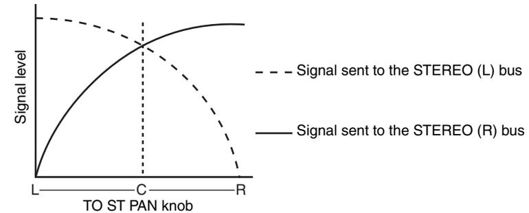
Operating the TO ST BALANCE knob of a STEREO channel will change the level of signals sent from the STEREO L/R channels to the STEREO (L/R) bus and MONO (C) bus, as shown in the following diagram. In this case, the TO ST PAN knob operates as a conventional BALANCE knob, and no signal is sent to the MONO (C) bus.
