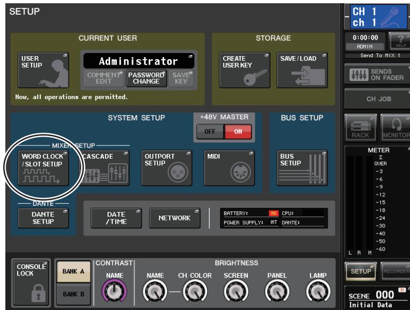
2. In the **SYSTEM SETUP** field at the center of the screen, press the **WORD CLOCK / SLOT SETUP** button to open the **WORD CLOCK / SLOT SETUP** popup window.
