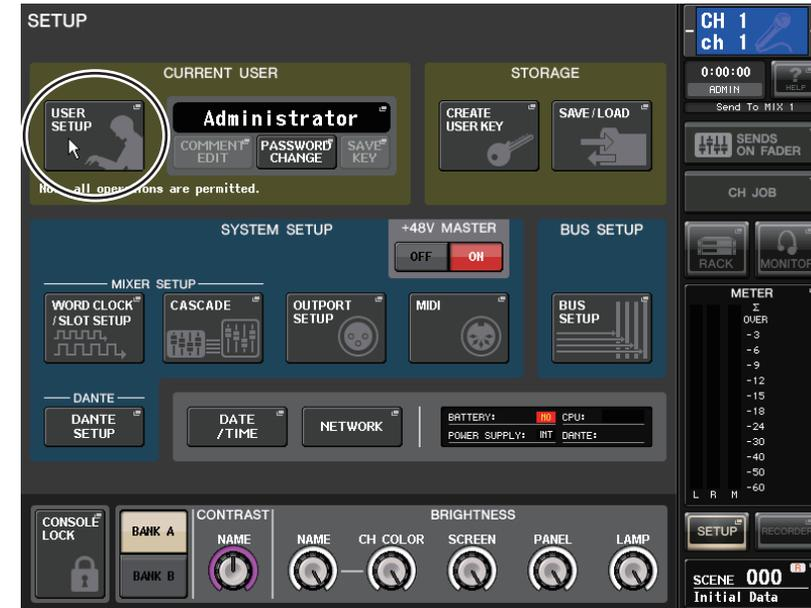
3. In the upper left of the screen, press the USER SETUP button to access the USER SETUP popup window.
