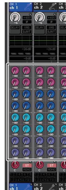
**7. Make sure that a MIX bus is selected as the send-destination in the TO MIX/TO MATRIX field.**
