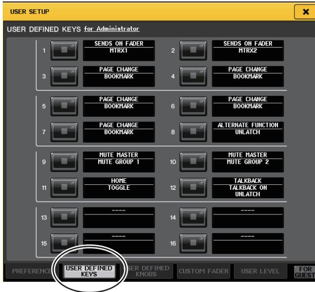
5. Press the button corresponding to the USER DEFINED key to which you want to assign the Help function.
