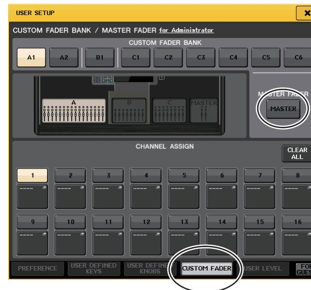
3. Press the CUSTOM FADER tab to access the CUSTOM FADER BANK/MASTER FADER page.
