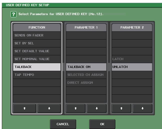
5. Make sure that the FUNCTION field is enclosed by a frame, then use the  $\uparrow/\downarrow$  buttons in the lower part of the field or the multifunction knobs on the top panel to select the function you want to assign.
