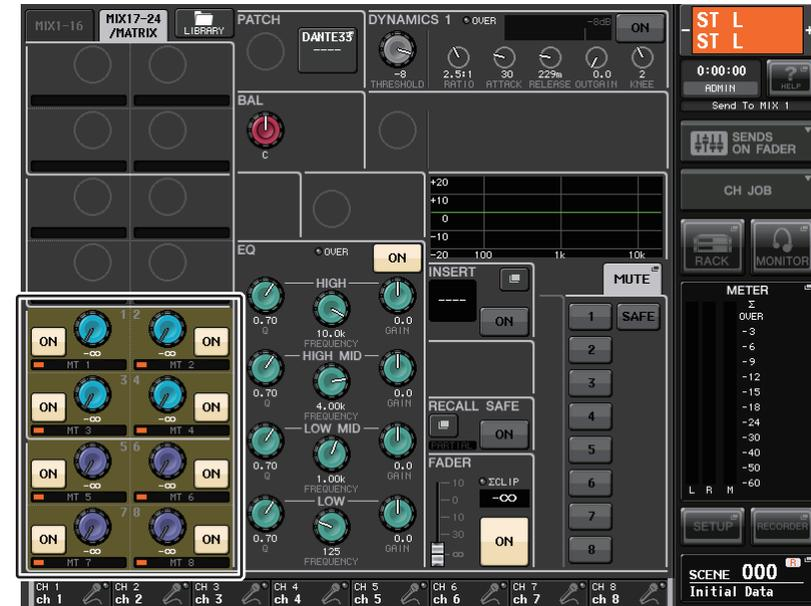
5. Make sure that the TO MATRIX SEND ON/OFF button is turned on for the send-destination MATRIX bus.
