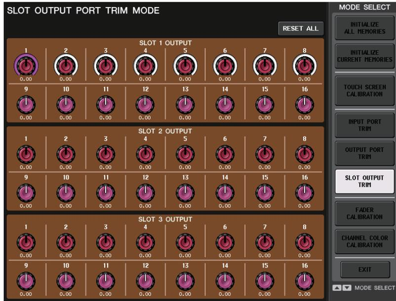
3. Press an on-screen knob to select it, and then use the corresponding multifunction knob to adjust the value.
