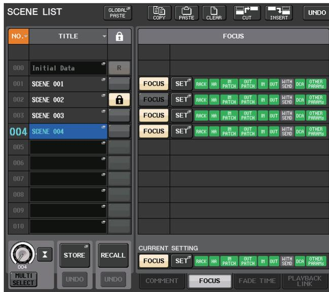
The FOCUS field enables you to make settings for the Focus function.
