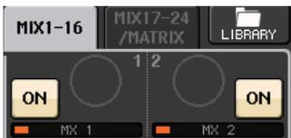
If the send-destination MIX bus is a VARI type, or if the send-destination is a MATRIX bus, the TO MIX SEND LEVEL knob will be displayed in the same color as the corresponding knob in the SELECTED CHANNEL section. In this case, you can use the corresponding knob in the SELECTED CHANNEL section to adjust the send level.
