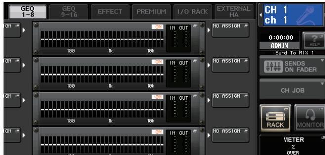
2. In the upper part of the VIRTUAL RACK window, press the GEQ 1-8, GEQ 9-16, or EFFECT tab to access the GEQ or EFFECT field.
