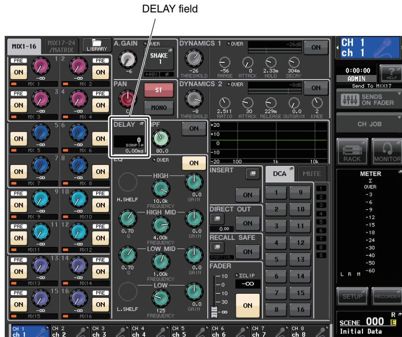
3. Press the DELAY field to access the DELAY popup window.
