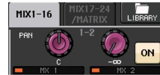
For a MONO channel, the right knob will adjust the common send level to the two MIX/MATRIX buses, and the left knob will adjust the panning between the two MIX/MATRIX buses. Rotating the left TO MIX/MATRIX SEND LEVEL knob counter-clockwise will increase the amount of signal sent to the odd-numbered MIX/MATRIX bus, and rotating it clockwise will increase the amount sent to the even-numbered MIX/MATRIX bus.
