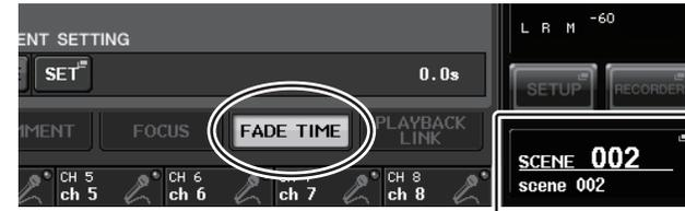
**2. Press the FADE TIME tab at the bottom of the SCENE LIST window.**
