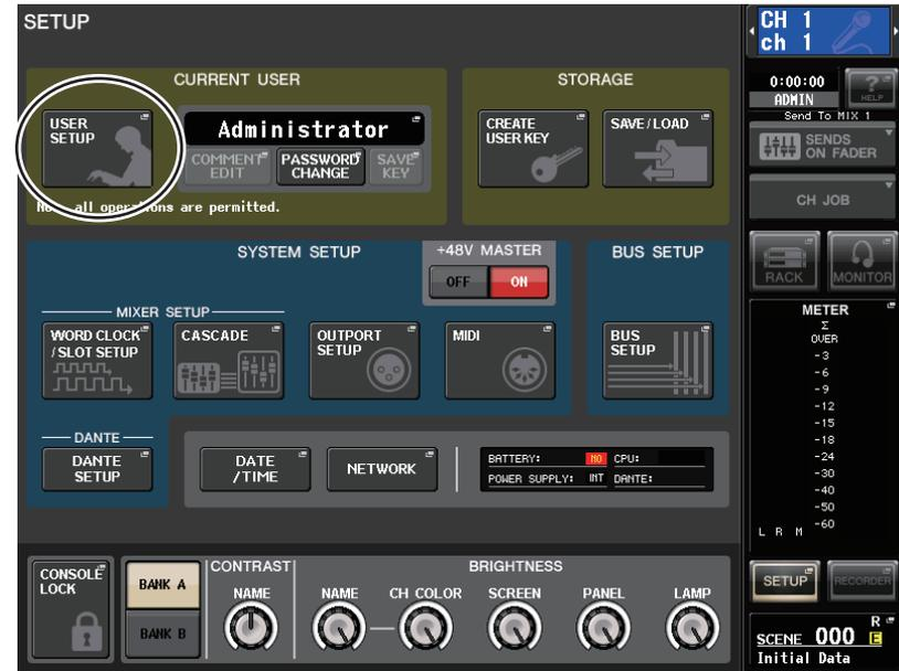
2. In the upper left of the screen, press the USER SETUP button to access the USER SETUP popup window.
