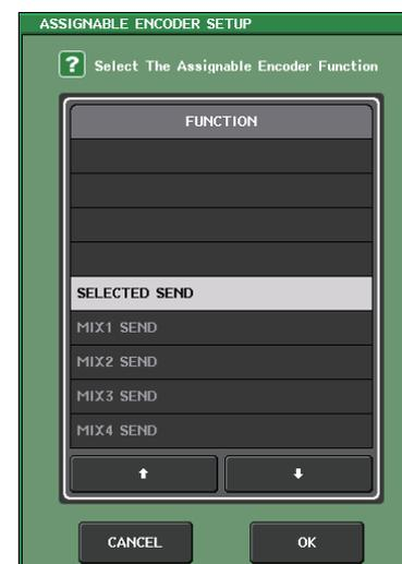
5. Use the **↑/↓** buttons in the lower part of the field or the multifunction knobs on the top panel to select the function you want to assign.
