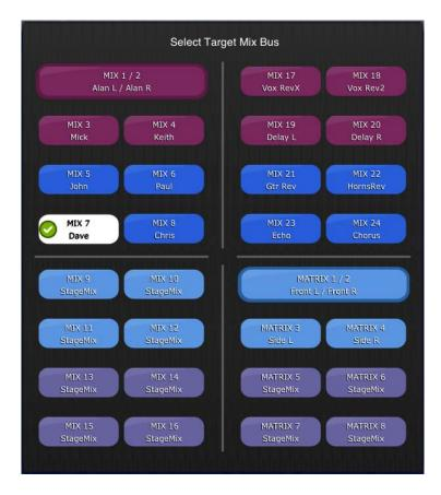
Choose the "Target Mix Bus" from Mix 1-24 and Matrix 1-8. The currently selected Mix will appear as a white button with a check mark. Stereo pairs appear as single large buttons.
