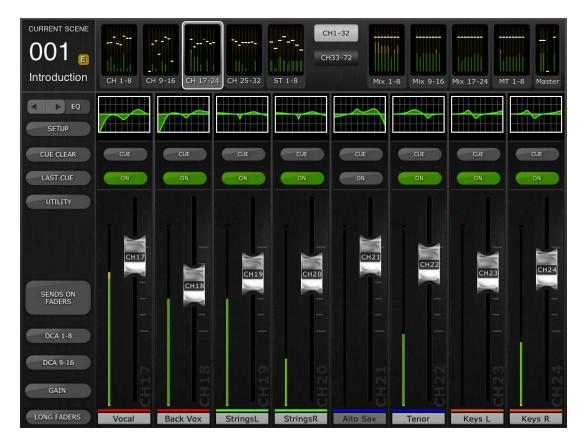
Across the top of the screen, level meters and faders are displayed in blocks of channels for mono Input Channels 1-32, Stereo Input Channels 1-8, Mix and Matrix busses, and the Master Stereo and Mono busses. This is the "Navigation/Meter Bridge".
