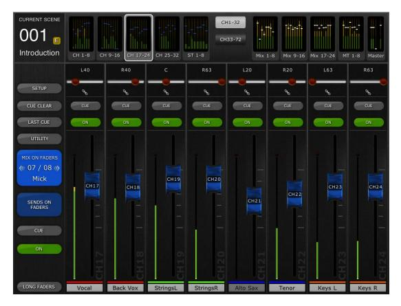
The large [MIX ON FADERS] button displays the currently selected Mix Bus number and its name. The color of this button matches those used in the series console.
