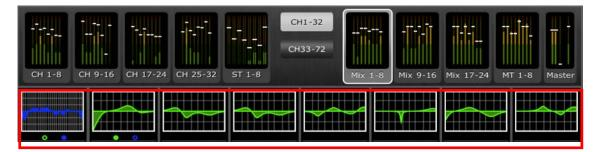
Green and blue dots below each EQ curve indicate the types of EQ available on that channel, and the type of EQ (PEQ or GEQ) that is currently displayed for that channel. A green dot indicates PEQ and a blue dot indicates GEQ. When only PEQ is currently available on a channel, no dots will appear below the curve. (In Demo mode, GEQs appear on Mix busses1, 7, 8, 12, 21 and Mono).
