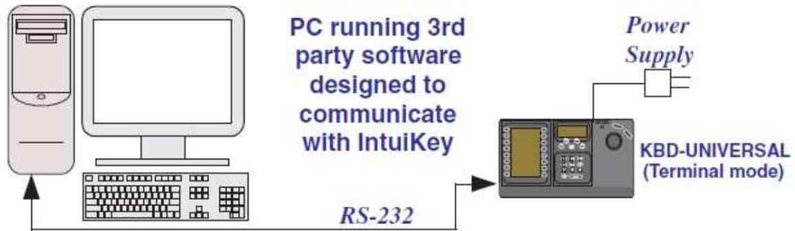
Figure 12: Keyboard connection.
