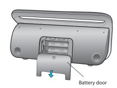
Slide the battery door off and insert 8 C cell batteries. Look for the + or symbols to put the batteries in correctly. Remember that the flat side of the
