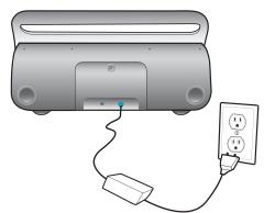
Plug the power adapter connector into the jack labelled "12V DC" and then to any 110 - 120V wall outlet or power source.
