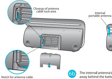
The internal antenna's connector and cable will be tucked away behind the battery door. Plug in the antenna. When sliding the battery door back into place be sure the cord exits through the small notch.
