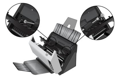
9. Rotate the lock tab into the scanner. Press down on the lock flange to lock the roller into the scanner.
