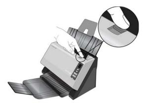
3. Wipe clean the feed rollers and scanner glass in the scanner body.
