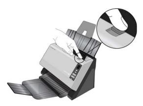
2. Squeeze the plastic clamps that hold the pad assembly in place and lift the pad up and out. Reverse the procedure to replace the new pad into its slots.
