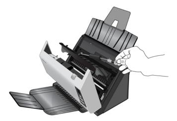
8. Angle the roller into the scanner and align the lock tab with the slot in the scanner.
