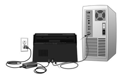
If the plug does not attach easily, make sure that you are plugging it in correctly. Do not force the plug into either connection.
