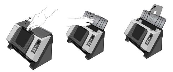
4. Pull the output tray down from the scanner body. It will snap in place when it is down all the way. Make sure the bottom of the tray is down all the way before scanning. If the tray isn't fully seated in position, paper feeding from the input tray may jam in the scanner.
