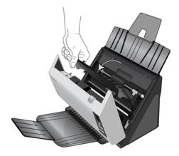
4. The roller is held in place with a lock tab that rotates to lock and unlock it. To unlock the tab, rotate it upward until the small lock flange is completely free.
