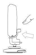
...THUMB LATCH RELEASED, BRACKET LATCH CLIPS RECEIVER SECURELY IN PLACE
