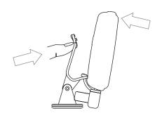
PLACE CAR BASE HOOKS INTO LOCKING SLOT & PUSH THUMB TAB IN...
