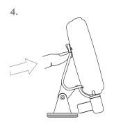
...ROTATE RECEIVER UNIT BACKWARDS TO ENGAGE HOOKS
