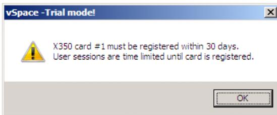
Reminder box displayed daily on each user station attached to an unregistered PCI card.
