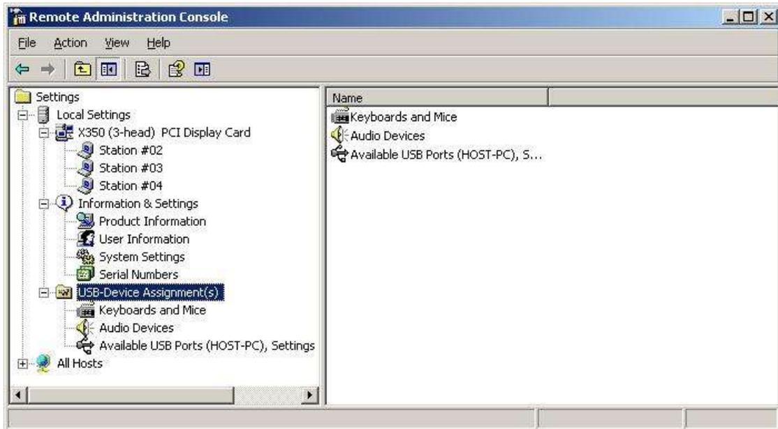
In the "USB-Device Assignment(s)" item, you can control which USB ports on the host PC are connected to which access device (station). To use this function, navigate the tree to select a connected USB device. After selecting a device, the following information will be displayed in the right-hand window.
