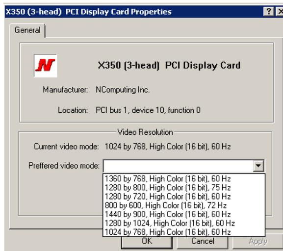
NOTE: Changing the PCI card's resolution and/or color depth is only allowed from the Administration console on the local system. Properties for cards inside other network systems can be remotely viewed, but resolution/color depth changes cannot be remotely applied.
