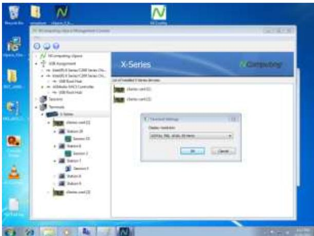
**Setting Screen Resolution:** You can set the screen resolution for all Stations connected to a PCI-card. To do this, click on the desired X-series PCI-card in the Terminals list. Right-click on the X-series card on the right side of the screen and choose “Terminal Settings” from the pop-up menu that is displayed. Choose the desired screen resolution from the drop-down menu and then click OK.
