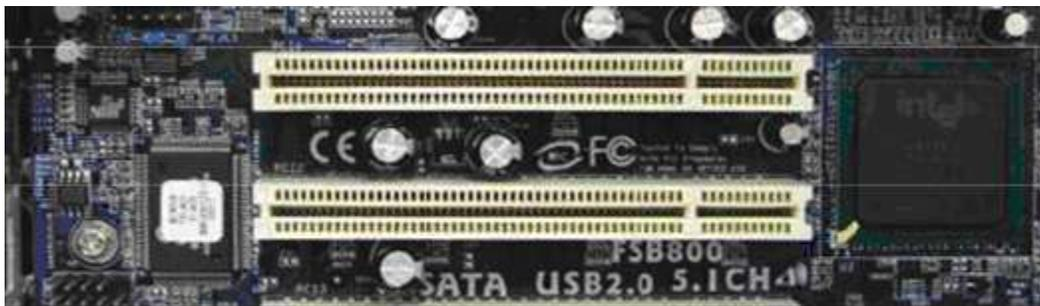
4. Insert one PCI card and secure the bracket to the chassis with a retaining screw (or other fastening mechanism specific to your PC). Note: The X550 is a full-height PCI card, and the X350 is a half-height PCI card.
