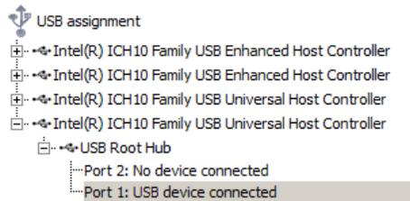
Expand the USB Assignment list to select a USB port on the host and configure it to be assigned to all stations, just the host or to a specific station.
