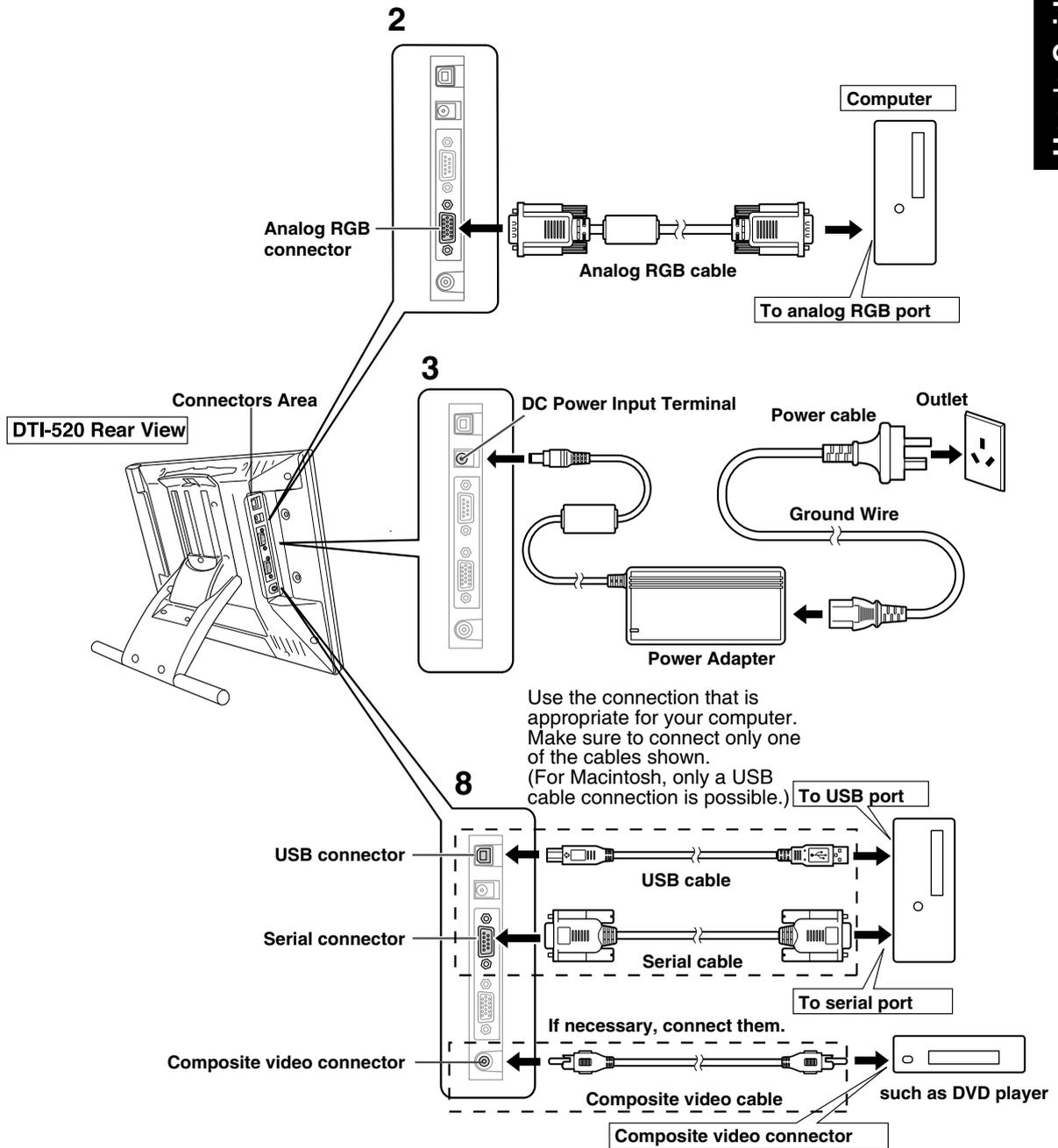
**Caution** When using the tablet with a serial cable connection, the product's USB hub function cannot be utilized.
