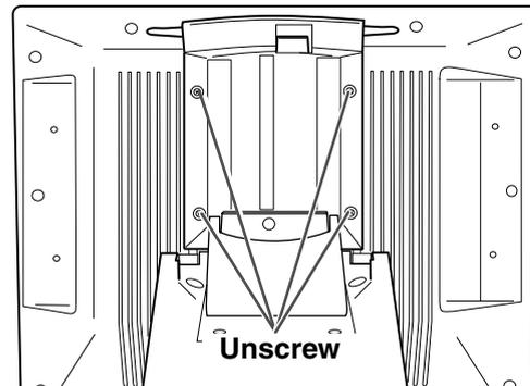
**4** Using four M4/0.7 mm screws, securely mount the arm or similar apparatus to the back of the unit.
