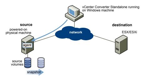
2 Converter Standalone prepares the virtual machine on the destination machine.
