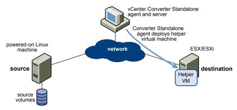
2 The helper virtual machine powers on, boots from the Linux image, connects to the source machine through SSH, and starts retrieving the selected data from the source. While you set up the conversion task, you can select which source volumes to be copied to the destination machine.
