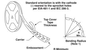
H Minimum: 8mm 1/2 Pitch and 8mm = .984" [25mm] 12mm, 12mm Double Pitch and 16mm =1.181" [30mm].
