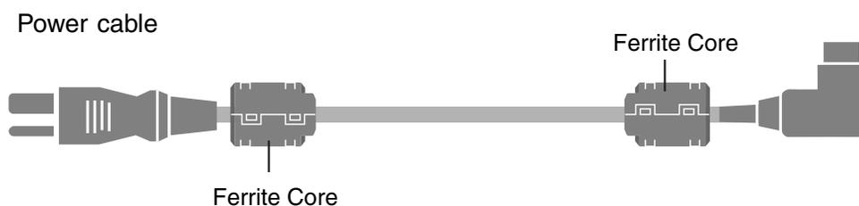
**Figure 4-1. Attaching the Ferrite Cores to the Power Cable**
