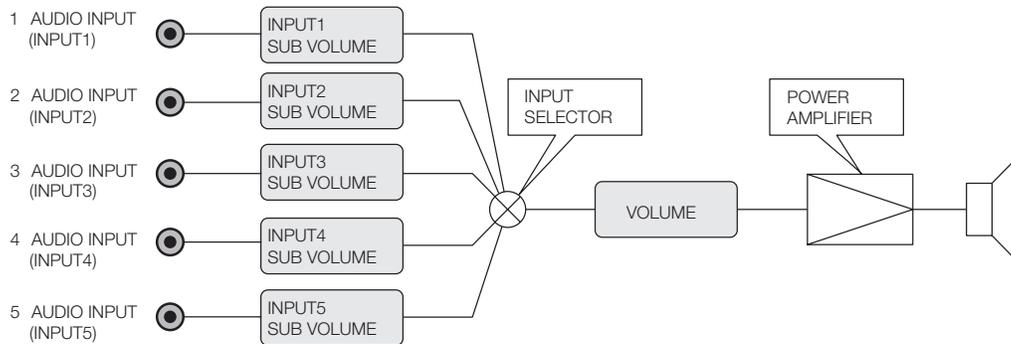
**Figure 4-7. Audio System Functional Block Diagram**
