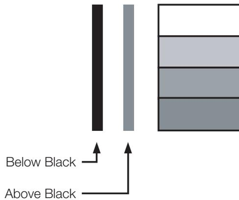
**Figure 4-3. Typical PLUGE Pattern for Adjusting Brightness**
