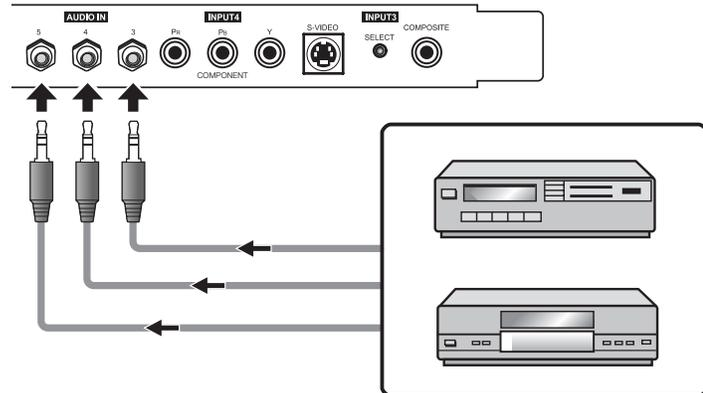
**Figure 3-10. Connecting Audio Inputs**
