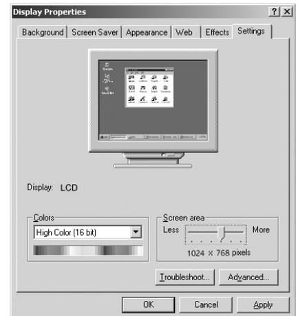
5. Click the **Advanced** button and click the **Monitor** tab on the dialog box. Set the vertical frequency to 60Hz and click **OK**.
