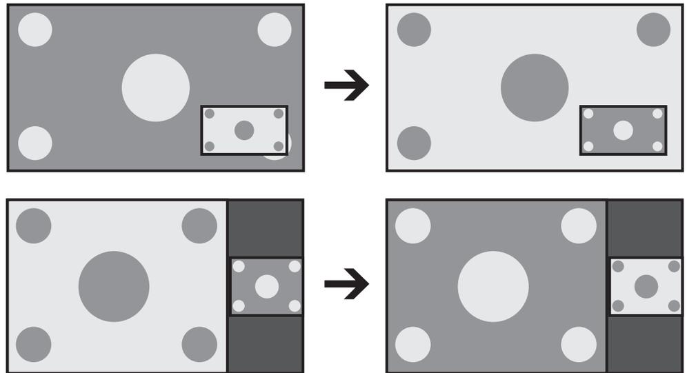
**Changing the PIP Position** ➤ To change the PIP window position, press the **PIP SHIFT** button on the remote control repeatedly until the window is in the desired position.
