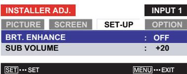
**Sub Volume (Installer Adjust mode):** Select **Sub Volume** from the Set-Up menu to adjust the audio input level for the current source. Do this for all sources, as needed to prevent sudden, drastic changes in sound volume when switching inputs.
