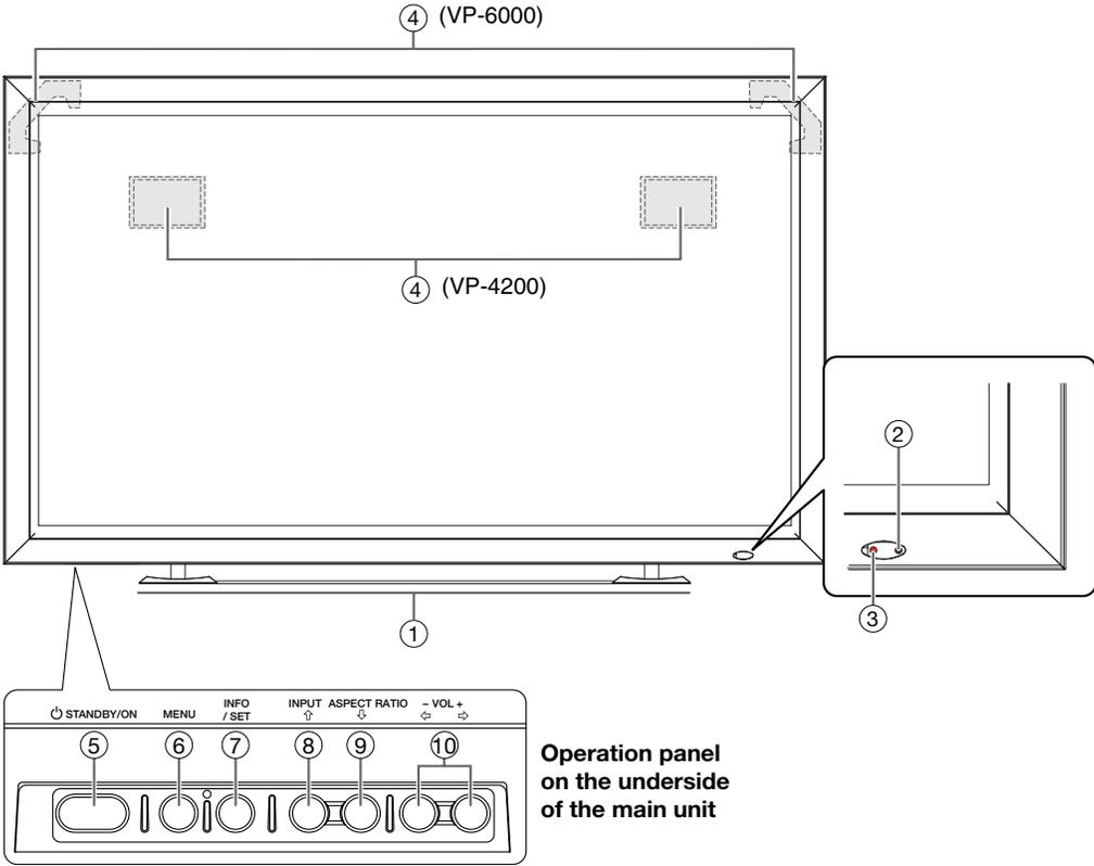
Operation panel on the underside of the main unit
