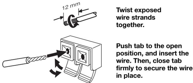
**Figure 3-12. Connecting Speakers**
