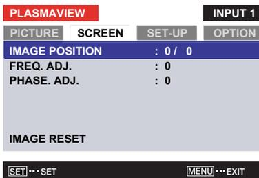
**Image Position:** Use the up- or down-arrow buttons (▲, ▼) to highlight **Image Position**. Then, press **SET** and use the left- and right-arrow buttons (◀, ▶) to shift the image horizontally; use the up- or down-arrow buttons (▲, ▼) to shift the image vertically.
