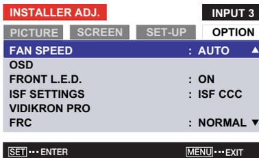
**Front L.E.D.:** Select **Front L.E.D.** from the Option menu to change the behavior of the front-panel STANDBY/ON indicator LED (Figure 2-1). When set to ON, the LED indicates operating status as follows:
