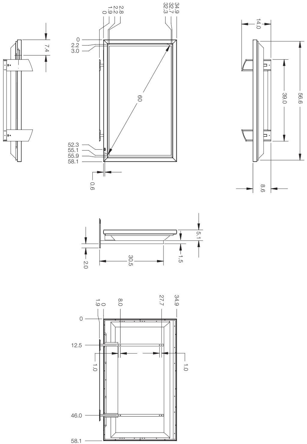
Figure 7-2. PlasmaView Model VP-6000 Dimensions (with Optional Table Stand)
