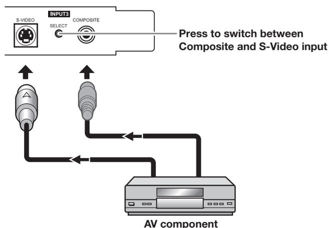
**Figure 3-6. Composite or S-Video (INPUT 3) Connection**
