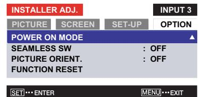
**Seamless Switch:** This feature allows for high-speed switching between any two PlasmaView inputs using the **SWAP** button on the remote control. To enable it, select **Seamless Switch** from the Option menu and set it to ON. Then, specify the two inputs you want to associate with this feature in the SELECT1 and SELECT2 fields.
