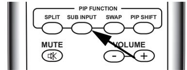
**Swapping the Main and PIP Windows** ➤ Press the **SWAP** button to replace the main screen with the sub-screen or vice versa. (This switches the audio input as well.)
