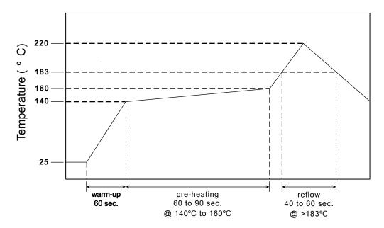
Note: EMXO's are precision subsystems with tolerances measured to  $\pm 0.001$  ppm. The EX-381/5 series has been designed for pick and place reflow soldering. The suggested reflow profile is shown above. The EX-381/5 may be reflowed one time in the non-inverted state. VI recommends waiting at least two hours after reflow before measuring the unit.
