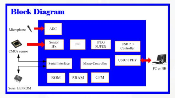
VC0332 is fully compliant with USB Video Class 1.0 standard and USB Audio Class 1.0 standard
