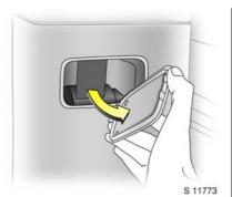
Should an interruption to the power supply occur, the fuel filler flap will not unlock in conjunction with the central locking \*. In such cases release manually.
