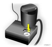
Reduce excess tyre pressure with the button above the pressure indicator.
