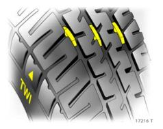
For safety reasons, tyres should be replaced when their tread depth has worn down to 2 to 3 mm. The legal permissible minimum tread depth (1.6 mm) has been reached when the tread has wom down as far as one of the wear indicators. A number of wear indicators are spaced at equal intervals around the tyre within the tread. Their position is indicated by markings on the tyre sidewall.
