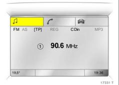
For each functional area there is a main page (Main), which is selected at the top edge of the display (not with the Infotainment system CD 30 or the Mobile Phone Portal):
