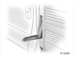
Pull the lever down until it contacts the body and lower the sideboard carefully.
