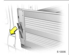
To lower the sideboard: Release both sideboard levers by pulling the lever outwards.
