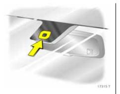
To ensure proper operation of the rain sensor \*, the sensor area must be free from dust, dirt and ice. The windscreen wash system must also be operated at regular intervals and the sensor area must be deiced. Vehicles with rain sensor \* can be identified by the sensor area near the top of the windscreen.
