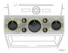
Vehicles without an air conditioning system do not have buttons for cooling 業, recirculation 经 or demisting and defrosting ም?.
