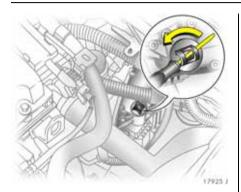
**Interruption of power supply** The clutch is not disengaged if the vehicle battery is discharged and a gear has been selected. The vehicle cannot move.
