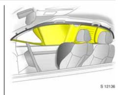
When the curtain airbag is triggered it inflates within milliseconds and provides a safety barrier in the head area on the respective side of the vehicle. This reduces the risk of injury to the head considerably in case of a side impact.
