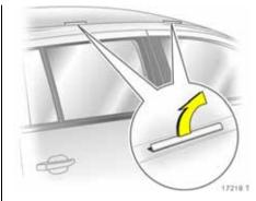
**Version without roof railing** Fold fitting opening covers upward.
