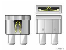
Only fit fuses of the specified current rating. Each fuse has its current rating written on it, in addition the ratings are colour coded.
