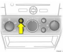
To activate/deactivate air conditioning compressor (cooling) 🌣 Operation only with engine running and fan switched off: ť٤
