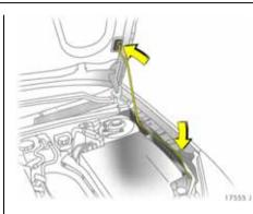
To hold the bonnet open, insert the support located on the left side in the small slot on the underside of the bonnet.
