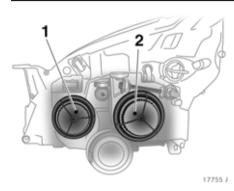
Halogen headlight system dipped and main beam
