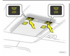
Front reading lights \* Left and right reading lights are individually operable. With ignition on:
