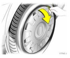
1. Prise off the wheel trim using the hook included with the vehicle tools. Vehicle tools – see page 235.
