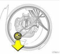
4. Remove parking light bulb holder from reflector.
