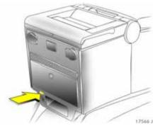
If it is correctly locked, the red mark must no longer be visible in the window, otherwise the procedure must be repeated.
