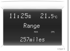
**Board information display** Display of time, outside temperature and date/infotainment system **\*** (when it is on).
