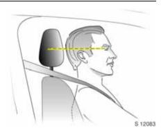
Head restraint position The middle of the head restraint should be at eye level. If this is not possible for extremely tall persons, set to highest position, and set to lowest position for small persons.
