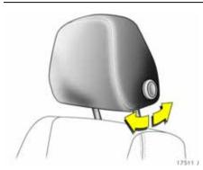
To adjust the incline, swivel the bottom edge of the head restraint forward or rearward
