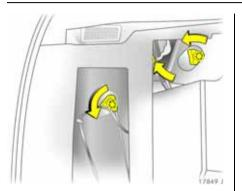
Hold bulb housing from outside, slacken fastening nuts using wheel bolt spanner \* and unscrew by hand. Remove bulb housing to rear. Wheel bolt spanner \* – see vehicle tools, page 235.
