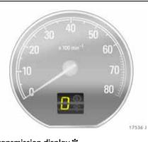
**Transmission display** Display of gear selected for automatic transmission **\*** or current gear or mode for Easytronic **\***.
