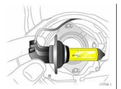
5. Remove the bulb holder with bulb from the reflector.
