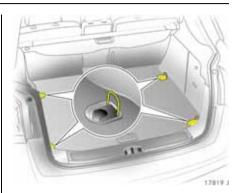
Lashing eyes In the luggage compartment, secure items being transported against slipping by attaching lashing straps \* or a luggage net \*.
