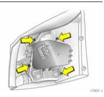
4. Press the retaining lugs on the outer edges of the bulb holder towards each other. Remove the bulb holder.
