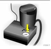
If the specified tyre pressure is not reached within 10 minutes, remove the tyre repair kit. Move the vehicle through one tyre rotation, approx. 2 metres, in either direction. Reconnect the tyre repair kit and continue the filling process for 10 minutes. If the specified tyre pressure is still not reached, the tyre is too badly damaged. Park the vehicle and contact a workshop.
