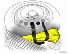
Towing equipment with removable coupling ball bar \* Stowage of coupling ball bar The coupling ball bar is stored in a bag strapped to the spare wheel.
