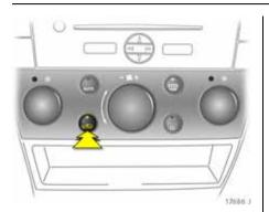
Manual air recirculation mode The air recirculation system prevents the entry of outside air and the air in the passenger compartment is circulated.
