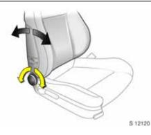
Adjusting the backrest To adjust, turn side handwheel on the seat while releasing the load on the backrest.
