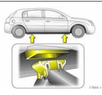
3. There are plastic retainers at the front and rear of the vehicle underbody for positioning the jack. The location of each retainer is indicated by a mark on the bottom edge of the vehicle.
