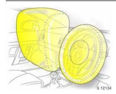
When triggered, the front airbags inflate in milliseconds to form a safety cushion for the driver and front passenger. The forward movement of the front seat occupants is checked, thereby substantially reducing the risk of injury to the upper body and head.
