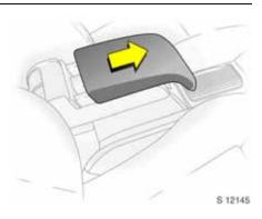
Armrest \* between the front seats The armrest can be pushed forward. If the armrest is not required, push it back and fold it up.
