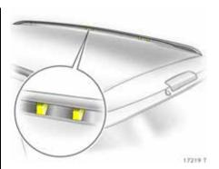
**Version with roof railing \*** Attach roof rack to roof railing at points shown in figure, see enclosed roof luggage rack system instructions.
