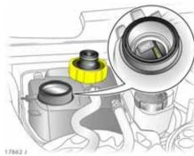
For V6 petrol and diesel engines, the expansion tank must be opened in order to check coolant level. When the cooling system is cold, the coolant should be up to the **COLD** mark on the filler opening.
