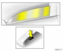
Closing windows from outside The windows can be closed from outside using the remote control: Depress the = button until the windows are closed.
