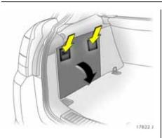
**Fuse box in luggage compartment** The fuse box is located on the left side of the luggage compartment, in the stowage compartment.
