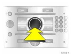
Selection using multifunction button: rotate and press multifunction button.
