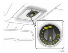
Operated using rotary switch in the overhead control panel.
