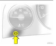
**Brake system control indicator** (D) The control indicator illuminates when the ignition is switched on if the hand brake is applied or if the brake or clutch fluid level is too low. Brake fluid – see page 272.
