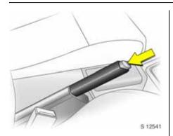
Releasing the hand brake: Raise lever slightly, press release button, lower lever fully ► Handbrake – see page 209.
