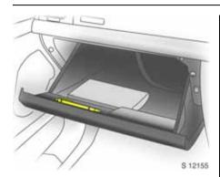
Stowage compartments Glove compartment To open, pull handle upwards.
