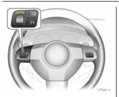
Selection using left-hand adjuster wheel on steering wheel: rotate and press adjuster wheel.
