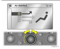
The individual menu items are marked by rotating the centre knob and selected by pressing it. Selecting certain menus by pressing the knob will open a submenu.
