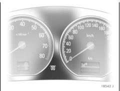
The control indicator  $\mathfrak{M}$  goes off as soon as the self-cleaning operation is complete.
