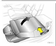
To move the rear seat backrest upright, pull handle on outboard side, move rear seat backrest upright and audibly latch.
