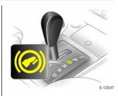
The engine can only be started with lever in position **P** or **N**. When position **N** is selected, press foot brake or engage hand brake before starting.
