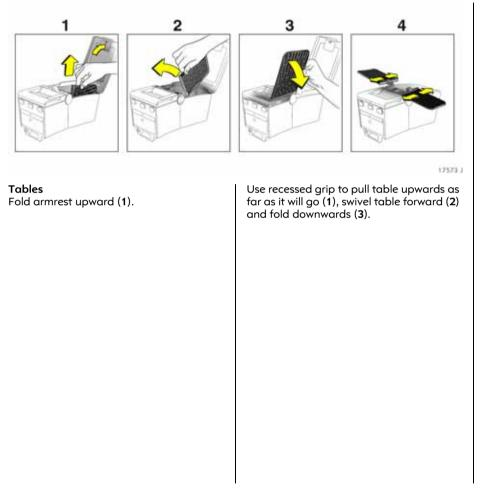
Set required clearance by adjusting longitudinal position of table (**4**).
