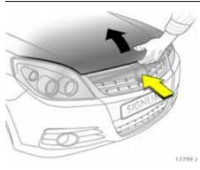
There is a safety catch on the underside of the bonnet: lift this upwards and open the bonnet.
