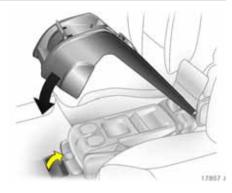
Swivel open and hold cover of front attachment points in floor in front of console.
