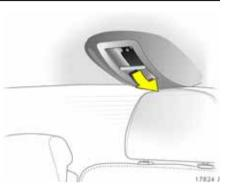
Three-point seat belt on centre rear seat Slide open cover in roof and remove seat belt latch plates from roof.
