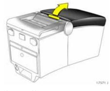
**Electric cool box** To open, fold open the armrest together with the stowage compartment. Switch on the cool box as needed.
