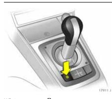
Winter program ☆ In the event of difficulties starting off on slippery roads, press button ☆ ("A" and ☆ appear in the transmission display). Easytronic switches to automatic mode and the vehicle sets off in second gear.
