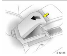
The armrest contains a stowage compartment: to open, slide armrest back, press button at front and lift.
