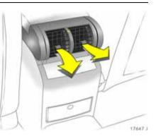
**Rear air vents \*** To open vent: Turn vertical adjuster wheel all the way up.
