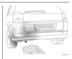
**Controlling exhaust emission** Some of the damaging substances in the exhaust such as carbon monoxide (CO), hydrocarbons (HC) and nitrous oxides ( $NO_x$ ) are reduced to a minimum by making structural changes – mainly in the injection system and the ignition system in conjunction with the catalytic converter.
