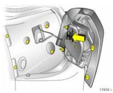
3. Detach cable plug from bulb housing.
