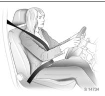
Adjust height such that the belt passes over the wearer's shoulder and rests against the shoulder. It must not pass over the neck or upper arm.
