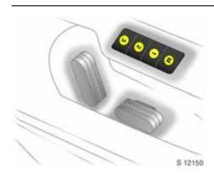
Memory function **\*** for electrically adjustable driver's seat and exterior mirrors
