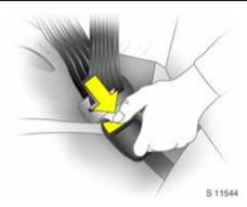
**Removing the belt** To release belt, press red button on belt buckle; the seat belt retracts by itself.
