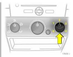
Air flow Setting with the right rotary switch.
