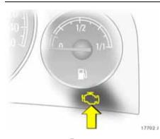
Control indicator <sup>(C)</sup> for exhaust Illuminates when the ignition is switched on and during the start attempt. Goes off shortly after the engine starts running.
