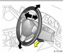
Steering wheel adjustment **\***: Move lever down, adjust height and distance, move lever up, engage
