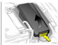
Disengage the bar at the front of the cover of fuse box and swing it upwards. Spare fuses, fuse extractor – see page 244. Some circuits may be protected by several fuses.
