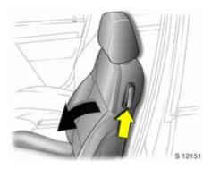
Folding down the front passenger seat \* Push head restraint on front passenger's seat down as far as it will go.
