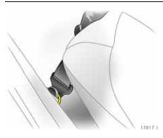
Hook belts into lashing eyes **\*** in floor behind front seats and tension.
