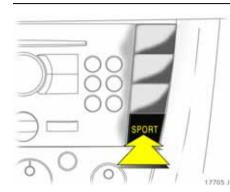
Damping and steering **\*** become more direct and provide better contact with the road surface. The engine reacts more quickly to accelerator movements.
