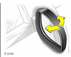
For the safety of pedestrians, the exterior mirrors will swing out of their normal mounting position if they are bumped with sufficient force. Reposition the mirror by applying slight pressure to the mirror housing.
