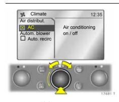
Activating and deactivating air conditioning compressor If no cooling or dehumidification is required, switch the air conditioning compressor off (maximum energy savings): Mark menu item AC from the manual settings menu and select by pressing. Eco appears on the display. Inflowing air is neither cooled nor dehumidified. This restricts the level of comfort provided by the electronic climate control system. This may cause the windows to mist up, for example.
