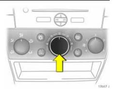
**Temperature preset** Setting with the centre rotary switch.
