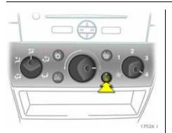
Heated rear window, heated exterior mirrors: On = Press () Off = Press () again
