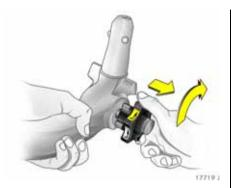
Otherwise, the coupling ball bar must be tensioned before it is inserted into the coupling housing: Open coupling ball bar.
