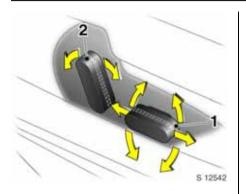
Adjusting the longitudinal position Move switch 1 forwards/backwards.
