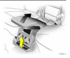
The underside of the centre seat cushion houses a console with stowage compartments and drink holders.
