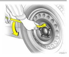
Turn wheel bolts half a turn using the wheel bolt wrench \*, pushing the wrench \* on as far as possible.
