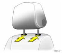
**Removing the head restraints** Press and release the two catches. Pull and remove the head restraint.
