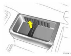
**Centre console stowage compartment \*** Division of the stowage compartment can be changed by moving the partition in the side guides. **Stowage compartment in the roof lining \*** To open, press the marked point.
