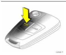
To deactivate Press button  $\geq$  of the remote control - or turn on the ignition.
