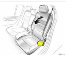
Adjusting backrest Pull handle at outboard side of seat and move backrest forward or backward. Release handle and allow seat to audibly latch.
