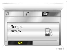
If less than 30 miles (50 km) can be driven with the fuel remaining in the tank, the warning "Range" appears on the display.
