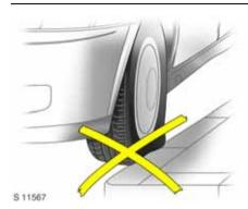
**Tyre condition, wheel condition** Drive over edges slowly and at a right angle if possible. Driving over sharp edges can lead to hidden tyre damage and wheel damage which is only noticed later on.
