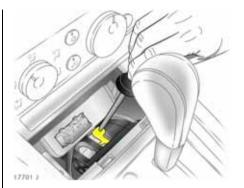
4. Push the yellow catch downwards with a screwdriver and move the selector lever out of **P**.
