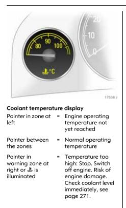
For physical reasons, the engine temperature gauge shows the coolant temperature only if the coolant level is adequate.
