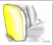
When triggered, the side airbag inflates within milliseconds to form a safety cushion for the driver or front passenger in the respective door area. This substantially reduces the risk of injury to the upper body and pelvis in the event of a side-on collision.
