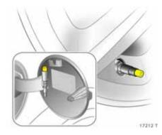
In vehicles with tyre pressure monitoring system **\*** there is an adapter in the valve cap key. Screw adapter to valve before attaching tyre pressure gauge, see page 204.
