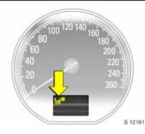
If the control indicator does not come on while driving, the front and side airbags for the passenger are not de-activated and there is a risk of injury or death to the child. Fit child restraint systems on the rear seat. Have the cause of the fault eliminated by a workshop.
