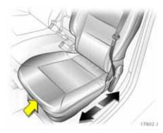
Rear seats Move seat Pull handle beneath seat and slide seat forward or backward. Release handle and allow seat to audibly latch.
