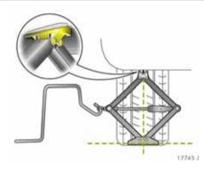
4. Before attaching jack \* set to required height by turning the eye by hand. Fit the jack \* at the front – or rear – in such a way that the jack head engages in the plastic retainer beneath the vehicle. Check that it is properly engaged.
