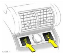
Heated rear seats \* Two switches at rear of centre console in front of the rear seats.
