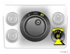
Headlight range adjustment © Manual headlight range adjustment \* With dipped beam switched on, adjust headlight range in four steps to suit vehicle load. Turn wheel against resistance and click it to the required position.
