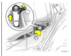
To change the lights on the left-hand side, remove filler neck from windscreen wash system bottle to gain better access: disengage retaining clamp and withdraw filler neck by pulling upwards. Wash fluid may escape if the bottle is full.
