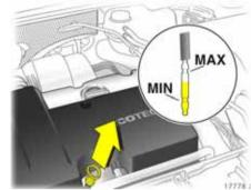
In vehicles with engine oil level monitoring **\***, the engine oil level is monitored automatically, see page 103. It is advisable to check the oil level before setting out on long journeys.
