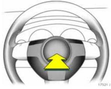
To operate horn: Press  $\bowtie$  in middle of steering wheel
