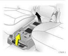
To fold out the seat cushion, pull handle beneath seat, lift at rear handle and tilt forwards by 180°.
