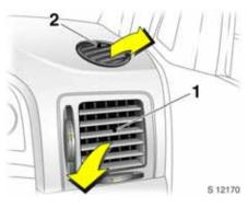
To close the vents turn the adjustment wheel fully downwards.
