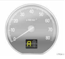
**Transmission display** Shows the mode or current gear.
