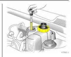
Antifreeze and corrosion protection Before the start of winter, have a workshop check the antifreeze protection. The antifreeze level must guarantee protection to approx. -28 °C. Insufficient antifreeze will reduce the frost protection level and the corrosion protection. If necessary add antifreeze.
