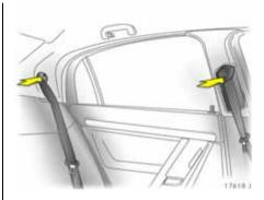
**Height adjustment** Height adjustment of upper anchorage point for front seat belts:
