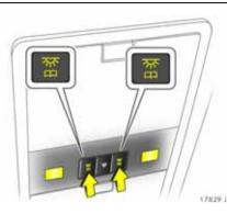
**Courtesy lights and rear reading lights** The rear courtesy light comes on at the same time as the front one.
