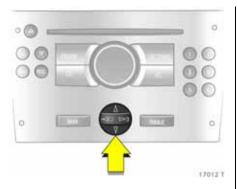
**To select with four-way button:** Select options via the menus and with the buttons/four-way button on the infotainment system **\***.
