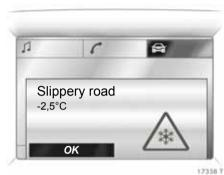
In vehicles with graphical information display **\*** or colour information display **\***, an icy road surface warning message appears in the display. No message is displayed if the temperature is less than -5 °C.
