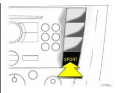
■ If the Continuous Damping Control is set to SPORT mode \*, the shift times are reduced and gear changes occur at higher engine speeds (not when cruise control is active). The control indicator \$ also illuminates in the transmission display, see page 176.
