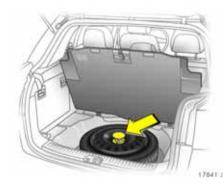
Remove protective cap and slacken wing nut. Remove spare wheel temporary spare wheel). The vehicle tools and the jack are beneath the spare wheel.
