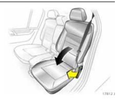
If fitted, remove the push-on sleeves **\*** for attaching the ISOFIX child restraint system **\***; see accompanying instructions for the ISOFIX child restraint system.
