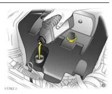
**Engine oil change, oil filter change** Change oil at a workshop according to the service interval shown on the display.
