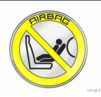
Vehicles with front passenger airbag can be recognised by the word **AIRBAG** above the glove compartment and the warning sticker on the sun visor of the passenger seat – see Fig. 17424 T. In some versions<sup>1)</sup>, the warning sticker may be on the side of the instrument panel – see Fig. 17118 T.
