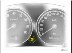
If the filter needs cleaning and recent driving situations did not allow the function to automatically operate, then the control indicator  $\mathfrak{M}$  will flash. If this occurs, then you may continue to drive the vehicle normally. The vehicle will not be damaged and does not require service.
