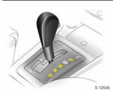
The selector lever can only be moved out of position  ${\bf P}$  or  ${\bf N}$  with the ignition switched on and the foot brake applied (selector lever lock). In selector lever position  ${\bf N}$  the selector lever lock is activated after a delay and only if the vehicle is stationary.
