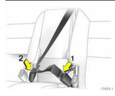
Engage lower latch plate into left-hand buckle (1) of the centre seat. Guide the seat belt by the upper latch plate over the shoulder and abdomen (avoid twisting) and engage in right-hand buckle (2) of the centre seat.
