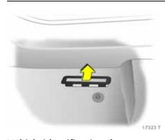
**Vehicle identification data** The vehicle identification number is stamped on the identification plate and beneath a cover on the floor of the vehicle between the front door and seat on the right-hand side. In other design variants, the identification plate may also be affixed to the dashboard.
