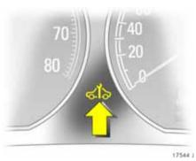
**Control indicator for immobiliser** Control indicator 소감> illuminates briefly when the ignition is switched on.
