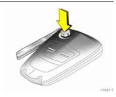
Key with foldaway key section \* Press button to extend. Press button to retract and audibly engage key section.
