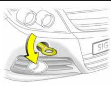
Screw in the towing eye anticlockwise as far as it will go until it stops in a horizontal position.
