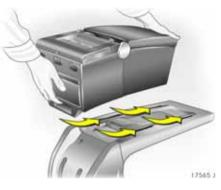
To lock, insert Travel Assistant into recesses in connecting console and slide back as far as possible.
