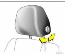
To adjust head restraint angle of front and outboard rear seats **\***: Swivel bottom edge of head restraint forward or rearward
