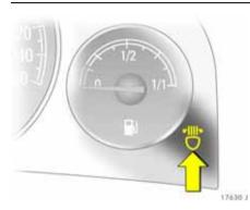
Control indicator ⊕ Flashing: Fault in system. The system is not ready for operation.
