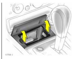
**Interruption of power supply** If the vehicle battery is flat, the selector lever cannot be moved out of position **P** or **N**.
