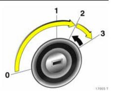
To start engine: Operate clutch and brake, automatic transmission \* in P or N, Easytronic \*: Depress brake, do not accelerate; Petrol engine: Turn key to 3; Diesel engine: Turn key to 2, when control indicator \$\mathcal{M}\$ goes out<sup>1)</sup>, turn key to 3; release key once engine is running
