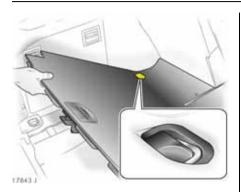
Stow away vehicle tools and jack – see page 235. Place defective wheel in spare wheel well with outside facing upward.
