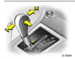
ActiveSelect (manual mode) Shift the selector lever from D first to the left and then forward or rearward.
