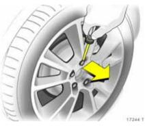
Alloy wheels \*: Disengage the wheel bolt caps with a screwdriver and remove. Protect the wheel by inserting a soft cloth between the screwdriver and ally wheel.
