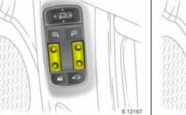
Operation via 2 rocker buttons in the driver's door. Additional rocker buttons in the front passenger door and the rear doors  $\overset{\bullet}{\ast}$ .
