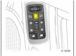
**Child safety system for rear windows \*** Switch 🗷 in the driver's door
