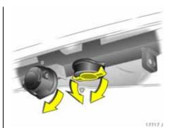
Fitting the coupling ball bar Compress the sealing plugs at the ends and pull out of the opening for the coupling ball bar. Stow the sealing plugs in the luggage compartment. Disengage socket and fold down **\***.
