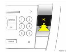
Activation without monitoring of passenger compartment and vehicle tilt Activate e.g. when animals are left in the vehicle.
