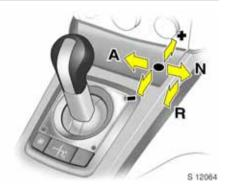
**Easytronic operation via the selector lever** Always move the selector lever in the appropriate direction as far as it will go. Upon release, it automatically returns to the centre position. Pay heed to the gear/mode indicator in the transmission display.
