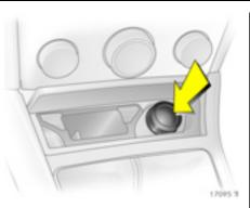
Press in cigarette lighter. Switches off automatically once the element is glowing. Pull out lighter.
