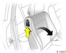
Tip the front seat backs forward \*: Lift release lever, tilt seat back forward.
