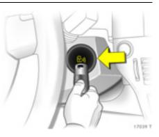
To start the engine, hold the electronic key at the marked position, depress brake pedal or clutch pedal or in vehicles with automatic transmission \* depress brake pedal and engage P or N, Then press the Start/Stop button.
