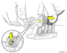
Join together the unfolded ends of the wind deflector: press in the pin at the slider, guide the hinge over the pin and release the slider so that the pin engages in the hinge.
