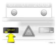
$\mathrm{ESP}^{\mathrm{Plus}}$  is reactivated by pressing the **SPORT** button again or switching on the ignition.
