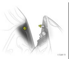
10. Insert the bulb housing in the body, engaging the lug and the ball pin in the recesses. Tighten the fastening nuts using a wheel bolt wrench \*. Attach the plug connector. Close and engage the flap.
