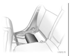
Remove the outer rear head restraints. Push the centre head restraint all the way down – page 88.
