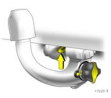
Lock coupling ball bar (key to position **2** – page 240, Fig. 17222 T). Remove key and press protective flap into position.
