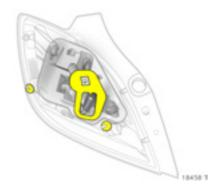
9. Ensure that the seals are applied to the bulb holder and fixing screws.
