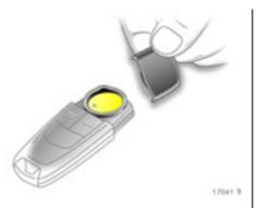
To replace the battery, press the locking mechanism on the underside of the electronic key and remove the cover towards the front by applying gentle pressure – page 73, figure 17037 T. Push off cover with emblem on the button side towards the outside.
