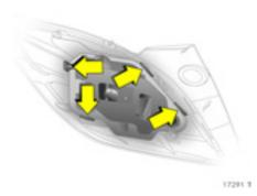
5. Remove the round seal from the fastening bolt. Press the locking tabs on the outside of the bulb holder outward and remove the bulb holder.
