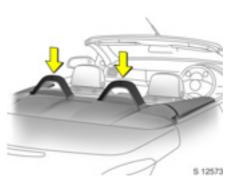
**Fixed anti-roll bars** are secured to the vehicle bodywork.
