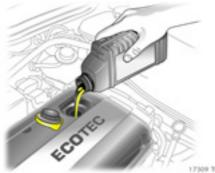
To check the engine oil level, insert wiped oil dipstick into handle as far as it will go. Top engine oil up if the level has dropped into the range of the top-up mark MIN.
