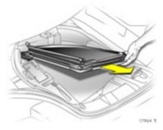
With tyre repair set \*, the wind deflector is folded down into a storage compartment \* in the luggage compartment below the loading floor cover.
