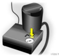
If the prescribed tyre pressure is not reached within 10 minutes. detach the tyre repair kit. Move the vehicle one tyre revolution (approx. 2 metres) in or against the flow of traffic. Reconnect the tyre repair kit and continue the filling procedure for 10 minutes. If the prescribed tyre pressure is still not reached, the tyre is too badly damaged. Park the vehicle and consult a workshop. We recommend your Vauxhall Authorised Repairer.
