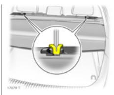
To cover the gap between the luggage compartment cover and the rear backrests, there is a cover on the cartridge. Attach the two hooks of the cover to the head restraint guide rods. If the safety net is mounted, run the hooks through the net mesh.
