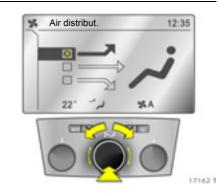
Individual menu items are marked by turning the centre knob and selected by pressing it. Selecting certain menus by pressing the knob will open a submenu **\***.
