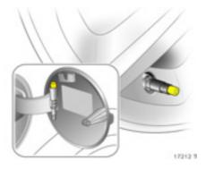
In vehicles with tyre pressure monitoring system **\*** there is an adapter in the valve cap key. Screw adapter to valve before attaching tyre pressure gauge – page 222.
