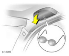
Stowage compartment for glasses \* On driver's side: fold down to open.
