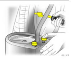
After having checked the tyre pressure, tighten the valve caps using the valve cap key.
