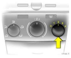
**Right-hand rotary switch: air flow** Four fan speeds:
