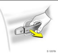
The electronic key must be within the external reception range about 1 metre from the vehicle in order to lock and unlock the vehicle.
