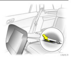
Raised seat cushions : Insert and adjust head restraints in backrests - pages 5, 88. Fold back seat cushions, making sure the belt buckles are properly positioned.
