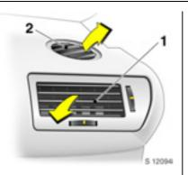
To close the vent, turn the vertical adjuster wheel fully up. The symbol **0** appears. The slats of the vent remain open although the air supply is closed.
