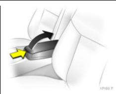
Stowage compartment in front armrest \* To open, press button and open upper part of armrest.
