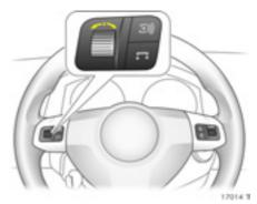
Selection with left adjuster wheel on steering wheel **\*** turn adjuster wheel and press.
