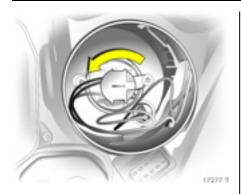
3. Rotate left bulb holder and disengage.
