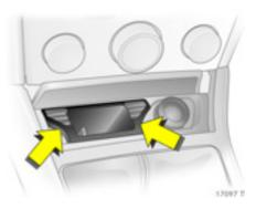
To empty, grip both sides of the ashtray insert at the spots illustrated and pull upwards.
