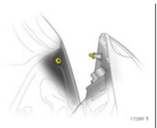
10. Insert the bulb housing in the body, engaging the lug and the ball pin in the recesses. Tighten the fastening nuts using a wheel bolt wrench \*. Attach the plug connector. Close and engage the flap.
