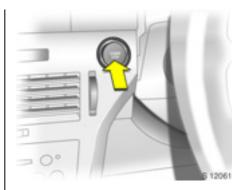
To start engine with Open&Start system **\***: The electronic key must be inside the car,
