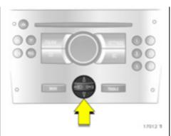
Select options via the menus and with the buttons/four-way button on the infotainment system **\***.
