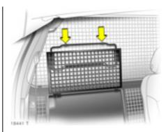
To close the grille section from the open position, press bracket down, fold down grille and lock.
