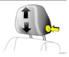
To adjust head restraint height of front and rear outboard seats: Press button to release, adjust height, engage in position
