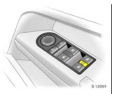
Child safety system for rear windows ☆ Switch ⊠ between the rear switches in the driver's door handle
