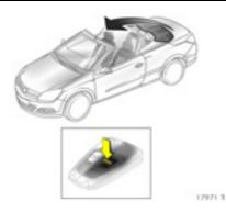
With the vehicle stopped, the roof can be closed using the radio remote control \*. Lock the vehicle. Press button — again and keep pressed until the roof and boot lid have closed completely.
