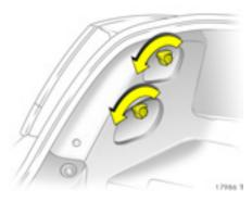
**Astra TwinTop** 1. Unscrew retaining nuts.
