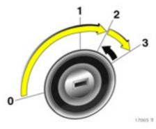
To start engine: Operate clutch and brake, automatic transmission \* in P or N,
