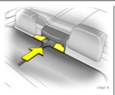
Insert the guide clips of the wind deflector in the seat belt recesses between the rear head restraints.
