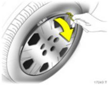
1. Prise off the wheel trim using the hook included with the vehicle tools \*. For vehicle tools, – page 256.
