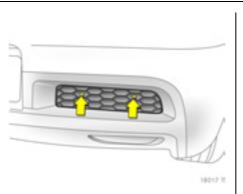
On some versions **\***: remove the cover concealing the towing eye at the rear right of the vehicle by disengaging the tabs at the bottom and pulling off the cover from the top.
