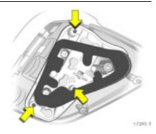
4. Unscrew the three screws with a screwdriver (vehicle tools – page 256) and remove the bulb holder.
