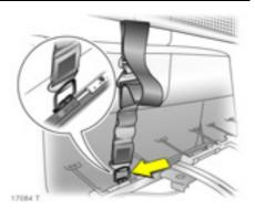
Adjustable rear row of seats **\***: Extend the safety net straps by adjusting the strap at the upper fastener in the loop of the strap (see Fig. 17085 T). Attach the straps in the brackets on the right and left raised seat cushions.
