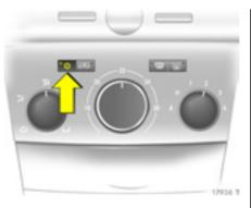
To activate/deactivate air conditioning compressor (cooling) Operate only with the engine on and the fan running: Press On= Press off= Constant again
