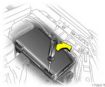
Fuse box in engine compartment The fuse box is at the front left side of the engine compartment.
