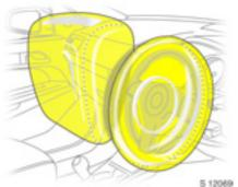
When triggered, the front airbags inflate in milliseconds to form a safety cushion for the driver and front passenger. The forward movement of the front seat occupants is checked, thereby substantially reducing the risk of injury to the upper body and head.
