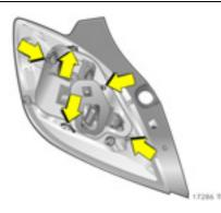
5. Unscrew three screws using a screwdriver (vehicle tools – page 256). Press locking tabs on outside of bulb holder inward and remove the bulb holder.
