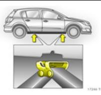
3. The location of each jacking point **\*** is indicated by a mark on the bottom edge of the vehicle.
