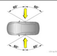
The curtain airbag system will be triggered:
