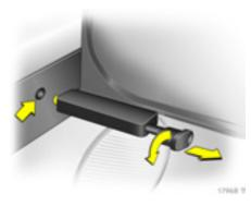
Pull the toggle of the right and left locking pin and turn to lock. Straighten out the wind deflector, turn the toggle back and engage the locking pin in the recess in the side trim.
