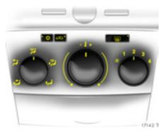
The buttons for cooling  $\overset{(*)}{\Rightarrow}$  and air recirculation  $\overset{(*)}{\Rightarrow}$  are only found on versions with optional air conditioning system  $\overset{(*)}{\ast}$ .
