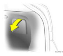
Hatch 3-door 1. To replace bulbs, fold the cover down.
