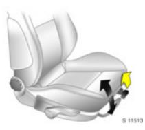
To adjust front seat inclination \*: Pull inner lever on front of seat, adjust inclination, release lever, engage seat in position
