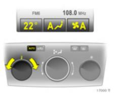
Set automatic mode on climate control system \*: Press AUTO, preselect temperature with rotary knob, open air vents
