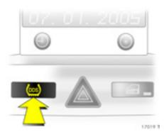
After tyre pressure is corrected or a tyre or wheel is changed, the system must be initialised by pressing the DDS button.
