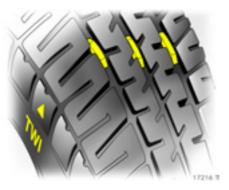
The legally permissible minimum tread depth (1.6 mm) has been reached when the tread has worn down as far as one of the wear indicators (TWI<sup>1)</sup>). A number of wear indicators are spaced at equal intervals around the tyre within the tread. Their position is indicated by markings on the tyre sidewall.
