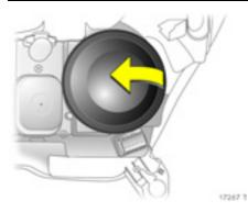
3. Rotate left bulb holder and disengage.
