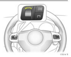
Depending on the equipment level of the vehicle, menu options can be selected with the left adjuster wheel \* on the steering wheel. The relevant menu options are then shown in order on the display.
