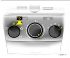
To demist or defrost windows: Set air distribution to **%**, rotary switch for temperature and air flow clockwise; Air conditioning system \*: also press button \$; Automatic air conditioning system \*: press button \$; and \$; turn rotary switch for temperature clockwise, air flow to A; Climate control system \*: press button \$?
