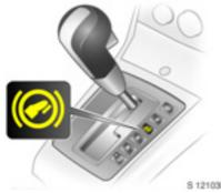
In position P or N, control indicator (S) illuminates red in the selector lever indicator strip if the selector lever is blocked.
