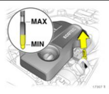
The engine oil level  $\overset{\bullet}{\ast}$  is checked automatically <sup>1)</sup>, see page 40. Before embarking on a long journey it is advisable to check the engine oil level.
