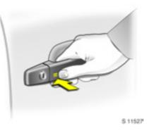
The vehicle is locked from the outside with the doors closed by touching the sensor panel in the door handle of one of the front doors. The electronic key must be within the external reception range of approximately one metre from the vehicle.
