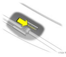
The vehicle identification number may be embossed on the instrument panel.
