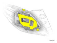
9. Ensure that the seals are applied to the bulb holder and fixing screws.
