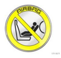
Use of child restraint systems **\*** on the front passenger seat in vehicles with airbag systems, but without seat occupancy recognition **\***
