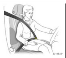
Fitting seat belt: Draw seat belt smoothly from inertia reel, quide over shoulder
