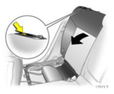
Disengage the backrest (single or split) using the sliders, fold it forward and engage.
