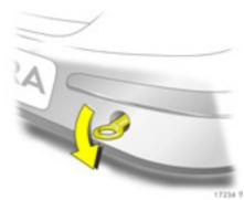
Screw in the towing eye anticlockwise as far as it will go until it stops in a horizontal position.
