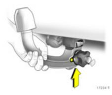
Inserting the coupling ball bar
