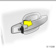
Only the driver's door can be locked and unlocked using the emergency key. Unlock the entire vehicle as described on page 80. In the version with Vauxhall alarm system \* the alarm may be triggered when the vehicle is unlocked. Switch ignition on to deactivate alarm and release the steering column lock: hold electronic key at marked position on the steering column panelling and press the Start/Stop button. Repeat procedure if necessary.
