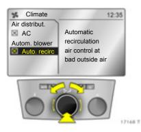
Switching automatic recirculation  $\ensuremath{\boldsymbol{\ast}}$  on or off
