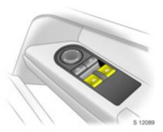
Operated via two or four \* switches in the driver's door handle. The front switches are for the driver and front passenger doors. The rear switches \* are for the rear doors. Additional switches are located in the front passenger door and rear doors \*.
