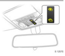
Central switch for electric windows, Astra TwinTop Button 4 or 4 in the roof console Press button 4 : all windows are closed Press button 4 : all windows are opened
