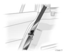
Restoring the backrests or seat cushions \* to their original position Guide the seat belts through the side brackets to protect against damage.
