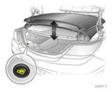
■ Briefly press button *C*: The folded roof is raised. The roof remains in this end position for approx. 9 minutes.
