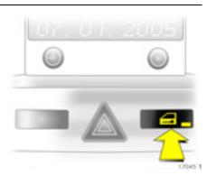
Central locking button for locking and unlocking the doors from inside the vehicle
