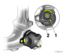
Checking the tensioning of the coupling ball bar
