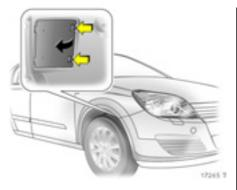
The bulbs of the front outer lights are replaced through openings in the front wheel arch: turn relevant wheels to gain access, release catch and remove cover.
