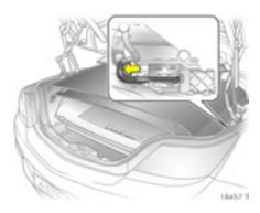
Unblocking on failure of electric drive Push locking lever forward as shown in the figure.
