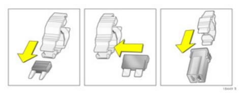
There is a fuse extractor in the luggage compartment fuse box to facilitate replacement of fuses - see figure above for an example. Place the fuse extractor on the various types of fuse from the top or side, and withdraw fuse.
