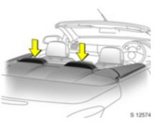
In the event of a rollover, the anti-roll bars deploy upwards in a matter of milliseconds. They also deploy together with the front and side airbag systems \*, helping to optimise occupant protection.
