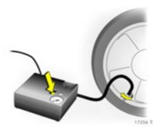
If tyre pressure is more than 1.3 bar, adjust to the prescribed value. Repeat the procedure until there is no more pressure loss.
