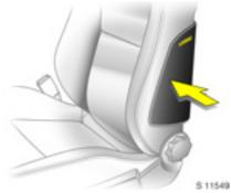
The side airbag system **\*** is identified by the word **AIRBAG** on the outboard sides of the front seat backrests.
