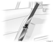
Restoring the backrests or seat cushions **\*** to their original position Guide the seat belt through the side bracket to protect against damage.
