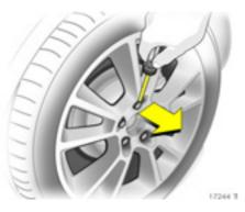
Alloy wheels \* : Disengage the wheel bolt caps with a screwdriver and remove. Protect the wheel by inserting a soft cloth between the screwdriver and ally wheel.
