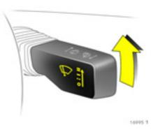
Automatic wiping with rain sensor \*: Move stalk upward -- = Automatic wiping with rain sensor
