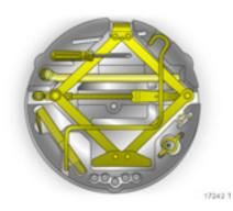
After use, stow away the jack and tools in the compartment as shown in illustration.
