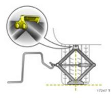
4. Before positioning the jack \*, set it to the necessary height by rotating the eye by hand. Position the jack \* at the front or rear so that the jack claw spans the vertical base and grips in the recess in the vertical base. Make sure it is properly positioned.
