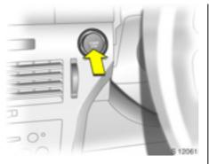
**Control indicator for immobilizer** রঠ Control indicator রঠ illuminates briefly when the ignition is switched on.
