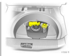
The tyre repair kit is in a compartment under the floor cover luggage compartment.
