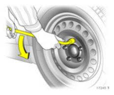
2. Turn wheel bolts half a turn using the wheel bolt wrench \*, pushing the wrench \* on as far as possible.
