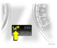
If the control indicator does not illuminate whilst driving, the front and side airbag **\*** have not been deactivated on the passenger side. Risk of fatal injury to the child - fit child restraint system to rear seat. Have cause of fault remedied. We recommend that you consult your Vauxhall Authorised Repairer.
