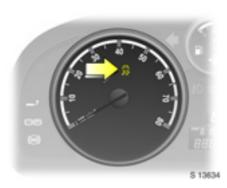
ESC Active & Warning control indicator The control indicator illuminates in yellow for approx. 4 seconds when the ignition is switched on. The system is ready for operation when it exting uishes.
