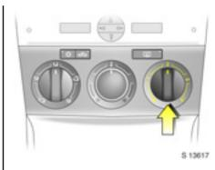
**Right-hand rotary knob: Airflow** Four fan speeds:
