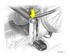
Attaching a bicycle to the Flex-Fix system Put on the bicycle. The pedal crank here must be placed in the pedal crank recess opening as shown in the illustration.
