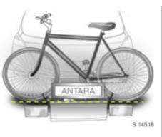
Place the wheel recesses such that the bicycle is more or less horizontal. Here, the distance between the pedals and the tailg ate should be at least 5 cm. Setting the wheel recesses - see page 154
