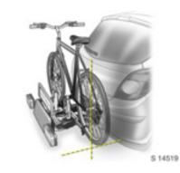
Align the bicycle in the longitudinal direction of the vehicle:
