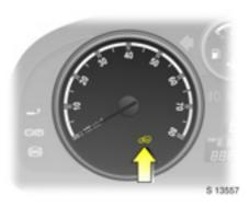
Control indicator for engine electronics Control indicator 🖙 illuminates for a few seconds when the ignition is switched on.
