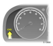
**Control indicator (D)(D) for brake system** Illuminates when ignition is switched on. Extinguishes after engine is started.
