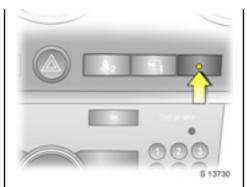
Confirm that the control indicator starts flashing slowly, after illuminating for approx. 30 seconds, to show that the antitheft system has been activated.
