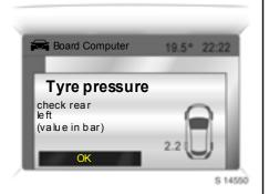
A graphic indicating the left rear tyre is shown together with the current tyre pressure; slight pressure deviation. Reduce speed. Check pressure at next opportunity with appropriate gauge and correct if necessary.
