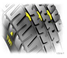
For safety reasons, tyres should be replaced when their tread depth has worn down to 2 to 3 mm. The leg al permissible minim um tread depth (1.6 mm) has been reached when the tread has worn down as far as one of the wear indicators.
