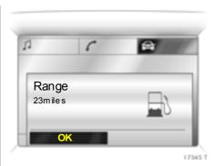
If the fuel in the tank will allow less than 30 miles (50 km) of travel, the warning "Range" appears on the display.
