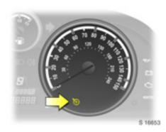
Control indicator for cruise control When driving, control indicator (3) will illuminate when the system is switched on and the desired vehicle speed is stored.
