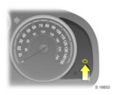
$\frac{\text{Control indicator for exhaust emissions}}{\text{Control indicator } \square \square \text{ illuminates for a few}}$  seconds when the ignition is switched on.
