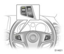
To select using the left adjuster wheel on the steering wheel:
