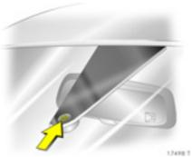
To ensure proper operation of the rain sensor \*, the sensor area must be free from dust, dirt and ice, which is why the windscreen wash system must be operated at regular intervals and the sensor area deiced. Vehicles with rain sensor can be identified by the sensor area near the top of the windscreen.
