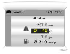
The information of the two trip computers can be reset separately, making it possible to evaluate data from different time period s.
