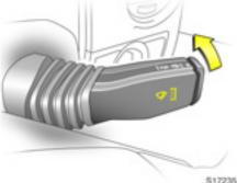
Automatic wiping with rain sensor \* To activate, move stalk upwards to automatic wiping with rain sensor position --.
