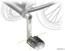
Prepare the bicycle for attachment Rotate the left pedal (opposite the chain cog) vertically downwards. The pedal on the left pedal crank must be horizontal.
