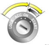
Starting the engine: Manual transmission in neutral, Depress clutch and footbrake, Automatic transmission in P or N, Do not accelerate
