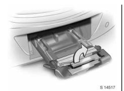
**Unfold pedal crank recesses**Fold one or both pedal crank recesses upwards until the diagonal support engages.
