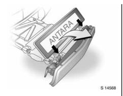
Pull up number plate holder and fully insert the holder supports into the retainers.
