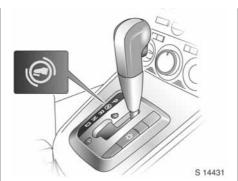
In position **P** or **N**, control indicator (S) illuminates in the selector lever indicator strip if the selector lever is blocked.
