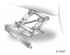
5. Attach wrench to eye of threaded rod and turn crank to raise vehicle.
