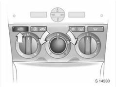
To set automatic mode of Electronic Climate Control \*: Press AUTO button, set temperature using rotary knob
