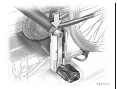
Attaching a bicycle to the Flex-Fix system Put on the bicycle. The pedal crank here must be placed in the pedal crank recess opening as shown in the illustration.
