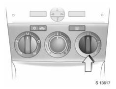
Right-hand rotary knob: Airflow Four fan speeds:
