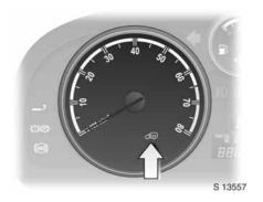
Control indicator for engine electronics Control indicator (29) illuminates for a few seconds when the ignition is switched on.
