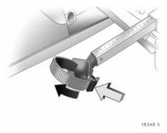
Push the release lever on the strap retainer and remove the strap retainer.
