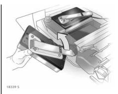
Open out the light support on the back of the tail light all the way.
