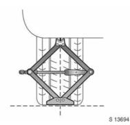
Before positioning the jack, set it to the necessary height by rotating the eye by hand.
