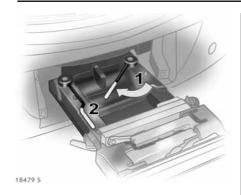
Swivel first the right clamping lever (1), inwards, followed by the left clamping lever (2), until they can be engaged in their respective recesses.
