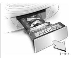
Completely pull out the Flex-Fix system until you hear it engage.
