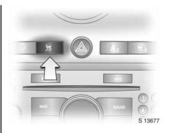
Turn off ESP function to allow engine rpm to increase, by pressing button  $\overline{\mathbb{R}}$ . Control indicator  $\overline{\mathbb{R}}$  illuminates in the instrument cluster.
