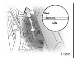
The illustrations show checking and replenishing the engine oil in the Z 24 petrol engineand the Z 20 diesel engines respectively.
