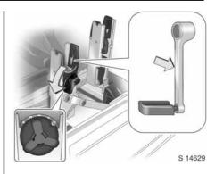
Adapting the Flex-Fix system to a bicycle With the rotary lever on the pedal crank recess, roughly adapt the adjustable pedal crank unit to the protrusion of the pedal crank.
