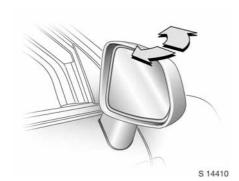
For the safety of pedestrians, the exterior mirrors will swing out of their normal mounting position in the event of an accident-like impact.
