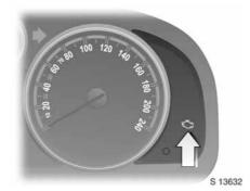
Control indicator for exhaust emissions Control indicator ♥ illuminates for a few seconds when the ignition is switched on.
