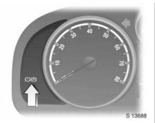
Control indicator (D)(D) for brake system Illuminates when ignition is switched on. Extinguishes after engine is started.
