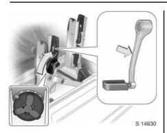
If the bicycle has curved pedal cranks, screw in the pedal crank unit all the way (position 1), see illustration.
