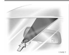
To ensure proper operation of the rain sensor \*, the sensor area must be free from dust, dirt and ice, which is why the windscreen wash system must be operated at regular intervals and the sensor area deiced. Vehicles with rain sensor can be identified by the sensor area near the top of the windscreen.
