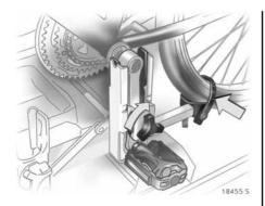
Tighten the attachment screw for the pedal bearing mount to its maximum point.
