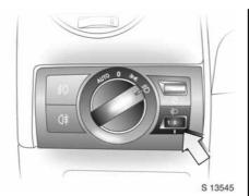
Headlight range adjustment \* With dipped beam switched on, adjust headlight range to suit vehicle load.
