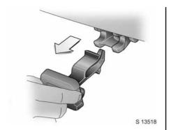
Fitting the coupling ball bar Remove sealing plug from the hole for the coupling ball bar and stow it in the luggage compartment.
