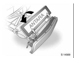
Pullup number plate holder and fold down into horizontal position.
