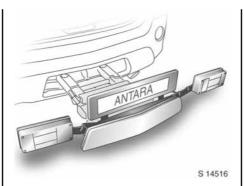
Check the cable and light position to make sure these are correctly installed and are securely located.
