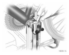
Insert pedal crank mount into outer rail of each pedal crank recess from above and slide downwards as far as it will go, see Fig. 18454 S on page 156.
