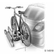
Align the bicycle in the longitudinal direction of the vehicle:
