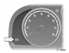
Control indicator (iii) for ABS Illuminates in yellow for approx. 4 seconds when the ignition is switched on.
