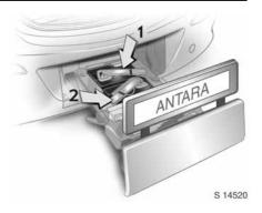
Fold in the light supports on the backs of the tail lights.
