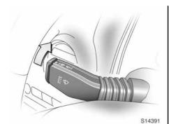
Automatic wiping with rain sensor \*
