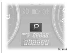
**Transmission display**Display of mode or current gear.
