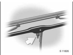
**Replacing windscreen wiper** Lift wiper arm, press and hold retaining clip and detach wiper blade.
