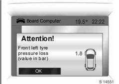
A graphic indicating the front left tyre is shown together with the current tyre pressure; significant pressure deviation or direct pressure loss. Steer out of flow of traffic as quickly as possible without endangering other drivers. Stop and check the tyres.
