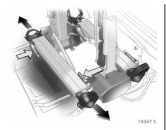
Press the release lever and withdraw the wheel recesses.
