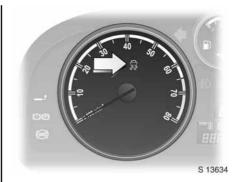
ESP Active & Warning control indicator The control indicator illuminates in yellow for approx. 4 seconds when the ignition is switched on. The system is ready for operation when it extinguishes.
