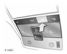
Courtesy lights can be turned off immediately by pressing button  $\dot{\Re}.$
