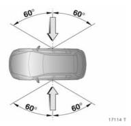
The side airbag system will be triggered:
