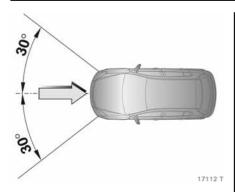
The front airbag system is triggered:
