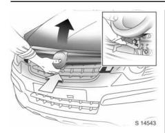
To open completely, locate the safety catch, found slightly left of centre on the underside of the bonnet, push the catch upwards and lift the bonnet gently. The bonnet is held open automatically.
