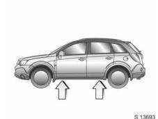
The location of front and rear jacking points is indicated by notches on the bottom edge of the vehicle, under the doors.
