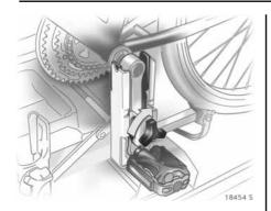
Attach the pedal crank by rotating the attachment screw on the pedal crank mount.
