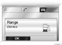
If the fuel in the tank will allow less than 30 miles (50 km) of travel, the warning "Range" appears on the display.
