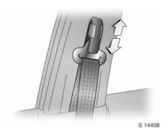
Seat belt height adjustment of front seat belt upper anchorage points
