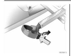
Secure the strap retainer and pull tightly downwards as far as possible.
