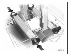
Press release lever and slide in wheel recesses all the way as far as they will go.
