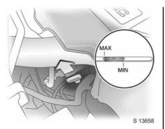
To check the level, remove dipstick from the dipstick tube, wipe it clean and re-insert it as far as it will go. After pulling the dipstick out again, check the oil level, ensuring it is between the lower and upper (or MIN and MAX) marks.
