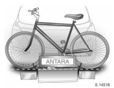
Place the wheel recesses such that the bicycle is more or less horizontal. Here, the distance between the pedals and the tailg ate should be at least 5 cm. Setting the wheel recesses - see page 154
