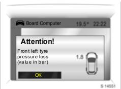
A graphic indicating the front left tyre is shown together with the current tyre pressure; significant pressure deviation or direct pressure loss. Steer out of flow of traffic as quickly as possible without endangering other drivers. Stop and check the tyres.
