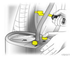
After having checked the tyre pressures, securely tighten the valve caps.
