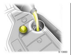
Engine oil level check and topping up
