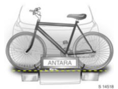
Place the wheel recesses such that the bicycle is more or less horizontal. Here, the distance between the pedals and the tailg ate should be at least 5 cm. Setting the wheel recesses - see page 155.
