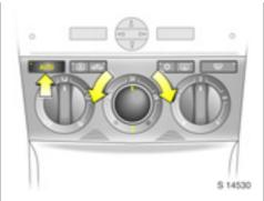
To set automatic mode of Electronic Climate Control \*: Press AUTO button, set temperature using rotary knob
