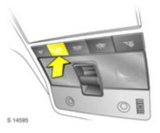
Activation without monitoring of passenger compartment and vehicle tilt \* Switch on when, for example, animals are to be left in the vehicle.
