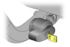
Lock coupling ball bar by turning the supplied key in the lock cylinder of the coupling ball bar.
