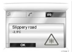
In vehicles with Graphical Information Display \* or Colour Information Display \*, a warning message appears on the display as a warning for icy road surfaces. There is no message below -5 °C.
