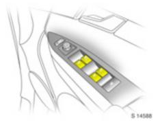
Operational with key in starter switch positions ACC or ON. If key is in LOCK position or removed, windows can be operated for 10 minutes or until driver's door is opened.
