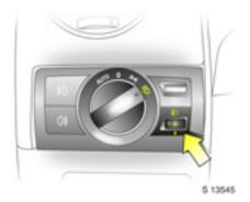
Headlight range adjustment \* Manual headlight range adjustment \* With dipped beam switched on, adjust headlight range to suit vehicle load.
