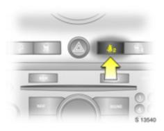
Front passenger's seat belt reminder \* \* Illuminates for approx. 4 seconds when ignition is switched on.
