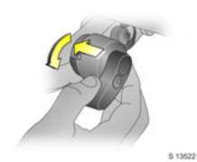
**Dismounting the coupling ball bar** Unlock coupling ball bar and remove key.
