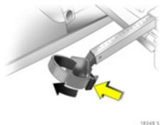
Push the release lever on the strap retainer and remove the strap retainer.
