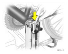
Insert pedal crank mount into outer rail of each pedal crank recess from above and slide downwards as far as it will go, see Fig. 18454 S on page 157.
