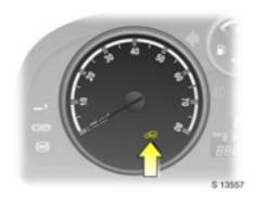
If it illuminates when the engine is running, there is a fault in the engine electronics. The electronics switch to the emergency running programme, fuel consumption may increase and the driveability of the vehicle may be affected.
