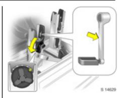
Adapting the Flex-Fix system to a bicycle With the rotary lever on the pedal crank recess, roughly adapt the adjustable pedal crank unit to the protrusion of the pedal crank.
