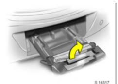
**Unfold pedal crank recesses**Fold one or both pedal crank recesses upwards until the diagonal support engages.
