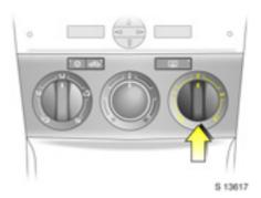
**Right-hand rotary knob: Airflow** Four fan speeds:
