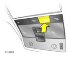
Courtesy lights can be tumed off immediately by pressing button  $\dot{R}$ .
