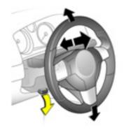
Steering wheel adjustment: Movelever down, adjust height and distance, move lever up and engage
