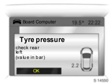
A graphic indicating the left rear tyre is shown together with the current tyre pressure; slight pressure deviation. Reduce speed. Check pressure at next opportunity with appropriate gauge and correct if necessary.
