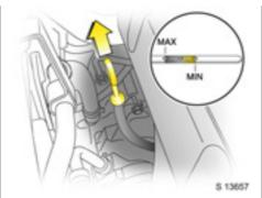
The illustrations show checking and replenishing the engine oil in the  $\it Z$  24 petrol engine and the  $\it Z$  20 diesel engine respectively.
