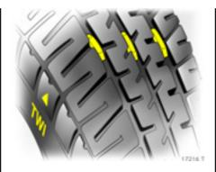
For safety reasons, tyres should be replaced when their tread depth has worn down to 2 to 3 mm. The legal permissible minimum tread depth (1.6 mm) has been reached when the tread has worn down as far as one of the wear indicators.
