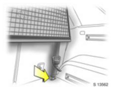
In front of and behind the rear seats on both sides of the vehicle are the hook holders (lashing eyes) for the lower strap hooks.
