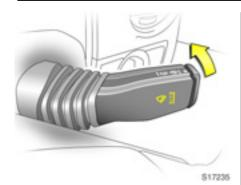
Automatic wiping with rain sensor \*
