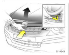
To open completely, locate the safety catch, found slightly left of centre on the underside of the bonnet, push the catch upwards and lift the bonnet gently. The bonnet is held open automatically.
