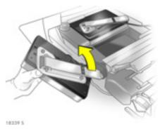
Open out the light support on the back of the tail light all the way.
