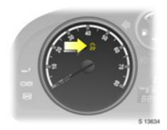
ESC Active & Warning control indicator The control indicator illuminates in yellow for approx. 4 seconds when the ignition is switched on. The system is ready for operation when it extinguishes.
