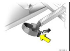
Secure the strap retainer and pull tightly downwards as far as possible.
