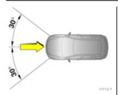
The front airbag system is triggered:
