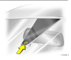
To ensure proper operation of the rain sensor \*, the sensor area must be free from dust, dirt and ice, which is why the windscreen wash systemmust be operated at regular intervals and the sensor area deiced. Vehicles with rain sensor can be identified by the sensor area near the top of the windscreen.
