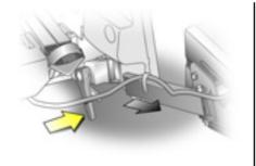
Push the clamping lever and pull both light supports out of the recesses.
