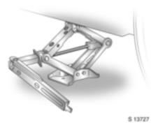
5. Attach wrench to eye of threaded rod and turn crank to raise vehicle.
