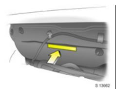
The Vehicle Identification Number (VIN) is also engraved on the top right-hand side of the bulkhead near the centre of the engine firewall.
