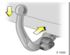
Inserting the coupling ball bar Insert the coupling ball bar into the coupling housing and push firmly downwards until the coupling ball bar audibly engages.
