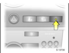
Confirm that the control indicator starts flashing slowly, after illuminating for approx. 30 seconds, to show that the antitheft system has been activated.
