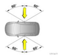
The side airbag system will be triggered:
