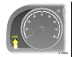
Control indicator (1)(1)(1) for brake system Illuminates when ignition is switched on. Extinguishes after engine is started.
