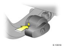
Confirm that the colour marking on the lever is red.
