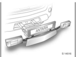
Check the cable and light position to make sure these are correctly installed and are securely located.
