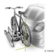
Align the bicycle in the longitudinal direction of the vehicle:
