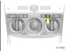
Heated rear window, heated exterior mirrors \*:
