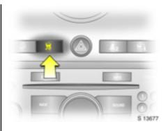
Turn off ESC function to allow engine rpm to increase, by pressing button  $\overline{\mathbb{R}}$ . Control indicator  $\overline{\mathbb{R}}$  illuminates in the instrument cluster.
