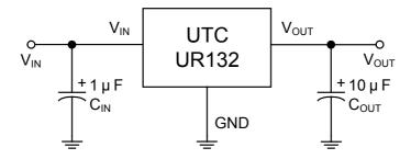
The part may oscillate without the capacitor, a  $10\mu$ F (or larger) capacitor is recommended between V<sub>OUT</sub> and GND for stability. Any type of capacitor can be used, but not Aluminum electrolytic when operating below -20°C. The capacitance may be increased without limit. Besides, another  $1\mu$ F capacitor (or larger) should be placed between V<sub>IN</sub> to GND.
