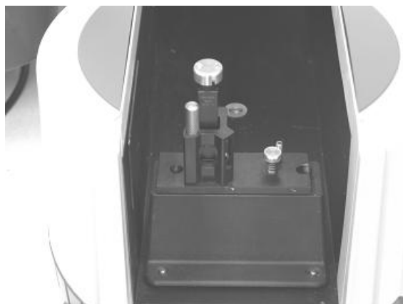
Figure 1. Cary 50 Bio UV-Vis spectrophotometer sample chamber fitted with a ultra-microvolume cuvette
