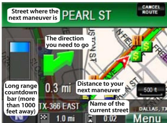
maneuver is further than 1000 feet away. At 1000 feet, it switches to the thousand-foot countdown bar.
