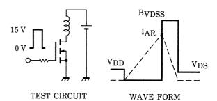
$$\begin{array}{l} T_{ch} = 25^{\circ}\text{C (Initial)} \\ \text{Peak I}_{AR} = 4.5 \text{ A}, \text{ R}_{G} = 25 \,\Omega \quad E_{AS} = \frac{1}{2} \cdot \text{L} \cdot \text{I}^{2} \cdot \left( \frac{\text{BVDSS}}{\text{BVDSS} - \text{V}_{DD}} \right) \\ \text{V}_{DD} = 24 \, \text{V}, \text{ L} = 1.0 \, \text{mH} \end{array}$$
