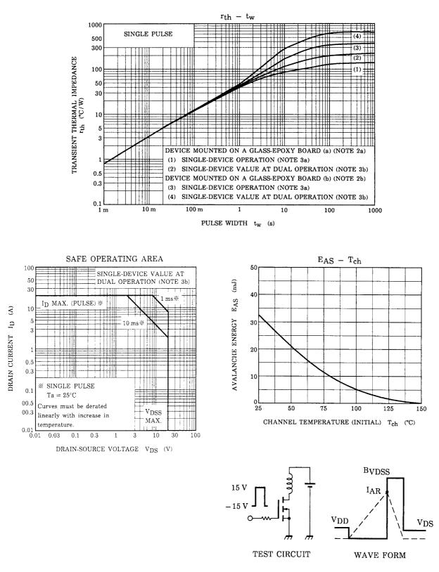
$\begin{array}{l} T_{ch} = 25^\circ C \ (Initial) \\ Peak \ I_{AR} = 5 \ A, \ R_G = 25 \ \Omega \quad E_{AS} = \frac{1}{2} \cdot L \cdot I^2 \cdot \left( \frac{B_{VDSS}}{B_{VDSS} - V_{DD}} \right) \\ V_{DD} = 24 \ V, \ L = 1.0 \ mH \end{array}$
