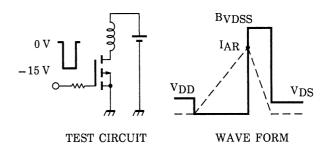
$$\begin{array}{l} T_{ch} = 25^{\circ}C \; (Initial) \\ Peak \; I_{AR} = -10 \; A, \; R_G = 25 \; \Omega \end{array} \quad E_{AS} = \frac{1}{2} \cdot L \cdot I^2 \cdot \; (\frac{BVDSS}{BVDSS - V_{DD}}) \\ V_{DD} = -24 \; V, \; L = 1.0 \; mH \end{array}$$
