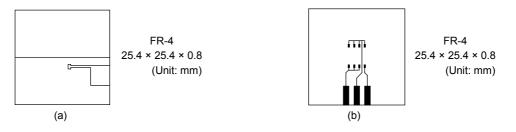
(b) Device mounted on a glass-epoxy board (b)
