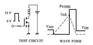
$$\begin{array}{ll} Peak~I_{AR}=7~A,~R_G=25~\Omega \\ V_{DD}=24~V,~L=1.0~mH \end{array} ~~E_{AS}=\frac{1}{2}\cdot L \cdot I^2 \cdot ~(\frac{BV_{DSS}}{BV_{DSS}-V_{DD}})$$
