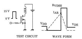
$$\begin{array}{l} T_{ch} = 25^{\circ}\!C~(Initial) \\ Peak~I_{AR} = 11~A,~R_G = 25~\Omega \end{array}~E_{AS} = \frac{1}{2} \cdot L \cdot I^2 \cdot ~(\frac{BVDSS}{BVDSS - VDD}) \\ V_{DD} = 24~V,~L = 1.0~mH \end{array}$$
