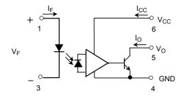
(Note) A 0.1µF bypass capacitor must be connected between pins 4 and 6.
