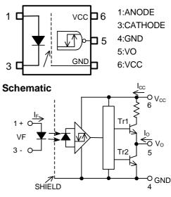
0.1uF bypass capacitor must be connected between pin 6 and 4
