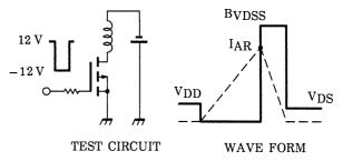
$$\begin{split} &T_{ch}=25^{\circ}C~(Initial)\\ &Peak~I_{AR}=-3.5~A,~R_{G}=25~\Omega~~E_{AS}=\frac{1}{2}\cdot L~\cdot I^{2}\cdot (~\frac{BVDSS}{BVDSS-V_{DD}})\\ &V_{DD}=-16~V,~L=1.0~mH \end{split}$$
