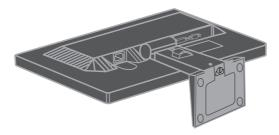
2. After placing the monitor face down on a clean surface or soft cloth, relax the bottom screws.
