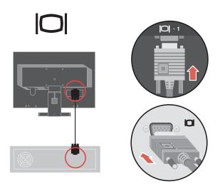
Connect the digital signal cable to the video port on the back of the computer. **Note**: One end of the signal cable is already pre-attached to your monitor.
