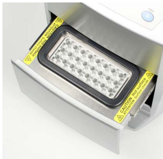
Figure 2–5. 24-well, max. volume 50 \mu l
