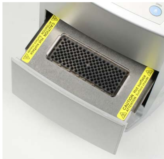
Figure 2–6. 96-well, max. volume 20 \mu l
