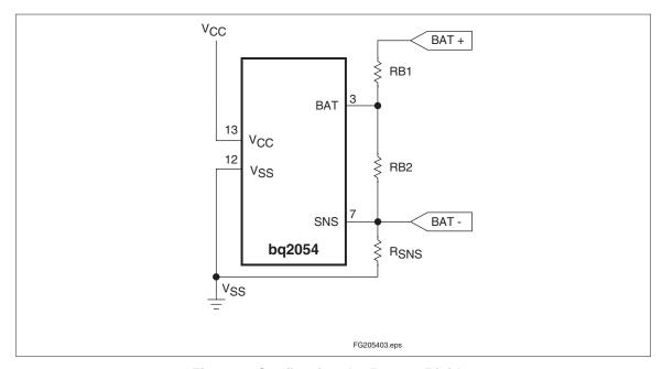
Figure 4. Configuring the Battery Divider
