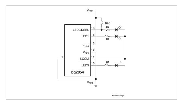
Figure 3. Configured Display Mode/IMIN Threshold
