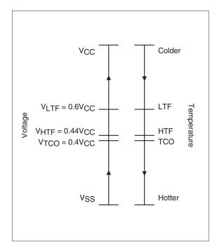
Figure 6. Voltage Equivalent of Temperature
