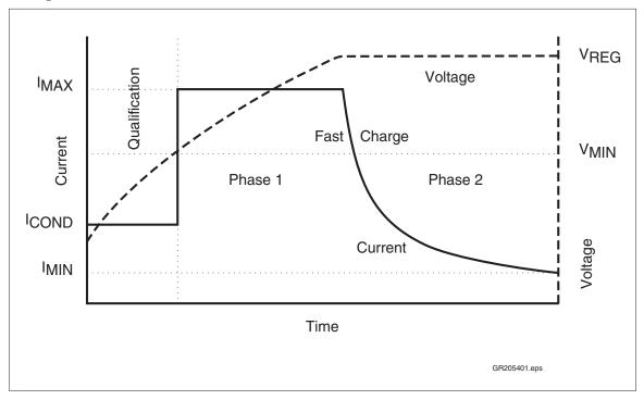
Figure 1. bq2054 Charge Algorithm
