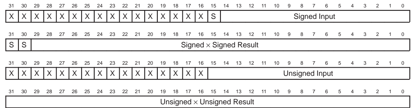
Figure 39. 16 x 16 Multiplier Data Formats
