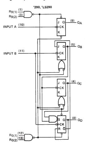
NOTES: A. Output  $Q_A$  is connected to input B for BCD count.
