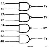
positive logic;  $Y = \overline{A \cdot B}$  or  $Y = \overline{A} + \overline{B}$
